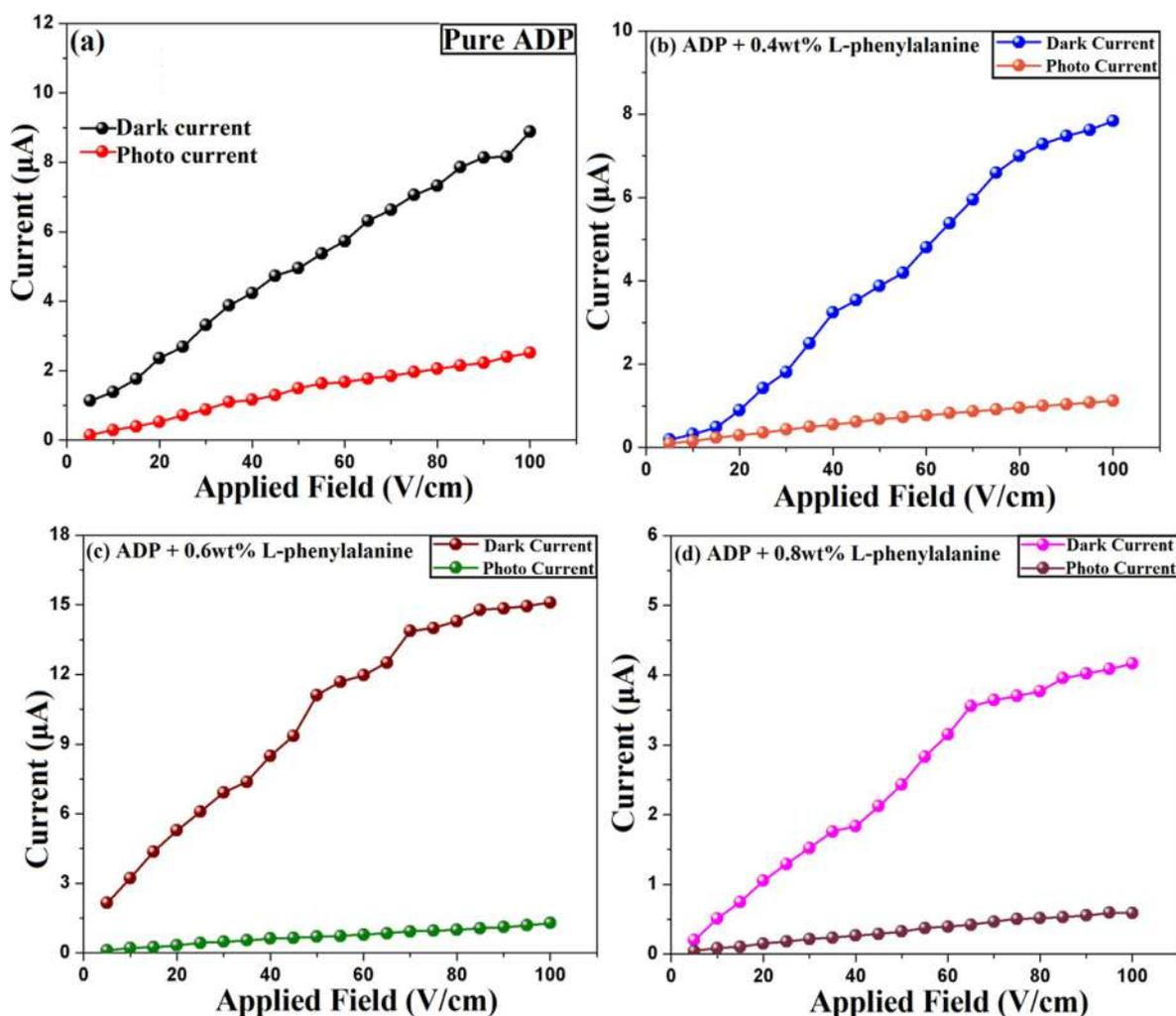
Fig. 6 (a-d). Photoconductivity spectra of pure and L-phenylalanine doped ADP crystal.
