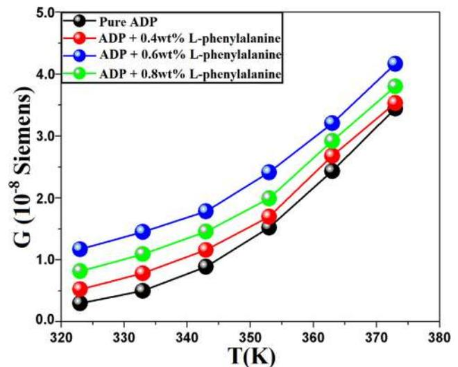
Fig. 9 Conductance versus temperature of pure and L-phenylalanine doped ADP crystals at  $\omega = 100 \text{ rad s}^{-1}$ .
