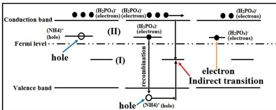
Fig. 7 Illustration of negative photoconductivity.
