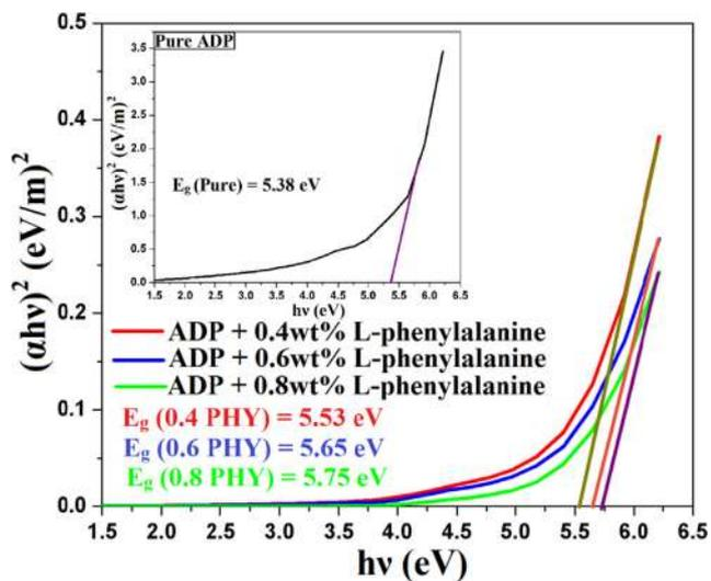
**Fig. 3** The tauc plot of pure and L-phenylalanine doped ADP crystals.
