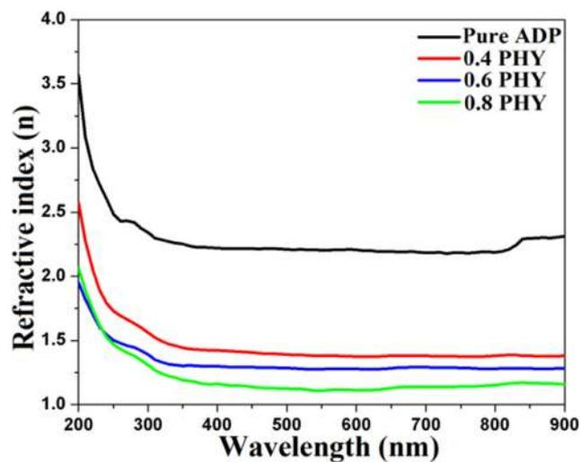
**Fig. 4** Refractive index spectra of pure and L-phenylalanine doped ADP crystals.
