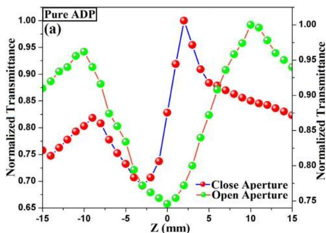
Fig. 10a Z-scan spectra of pure ADP crystal.
