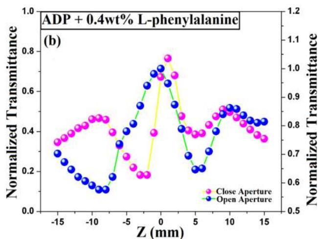
Fig. 10b Z-scan spectra of 0.4 wt% L-phenylalanine doped ADP crystal.
