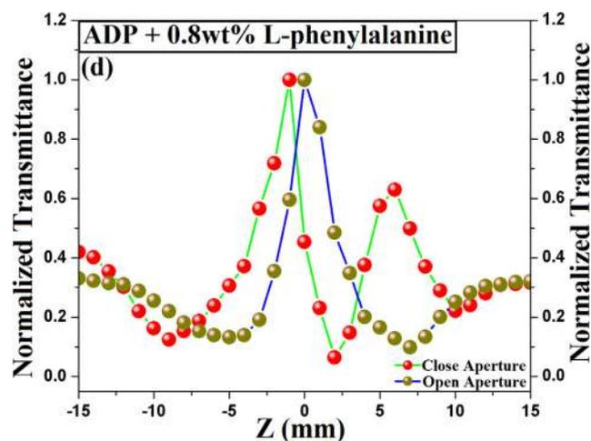
Fig. 10d Z-scan spectra of 0.8 wt% L-phenylalanine doped ADP crystal.
