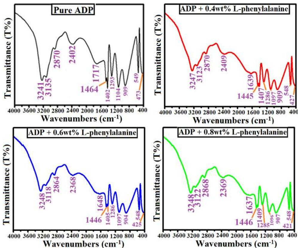
Fig. 1 FT-IR spectra of pure and L-phenylalanine doped ADP crystals.
