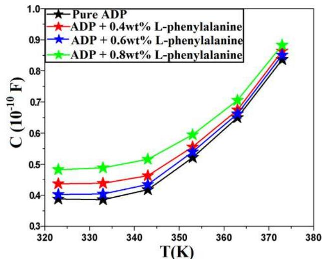
Fig. 8 Capacitance versus temperature of pure and L-phenylalanine doped ADP crystals at  $\omega = 100 \text{ rad s}^{-1}$ .
