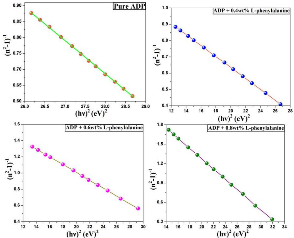
Fig. 5 (a-d). Refractive index dispersion plots for pure and L-phenylalanine doped ADP crystal.
