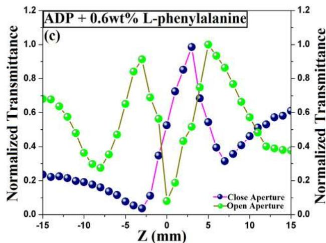
Fig. 10c Z-scan spectra of 0.6 wt% L-phenylalanine doped ADP crystal.
