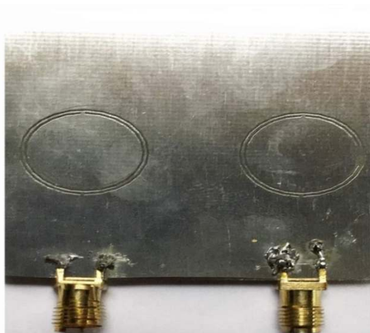
Figure 6: Fabricated antenna (b) bottom layer.
