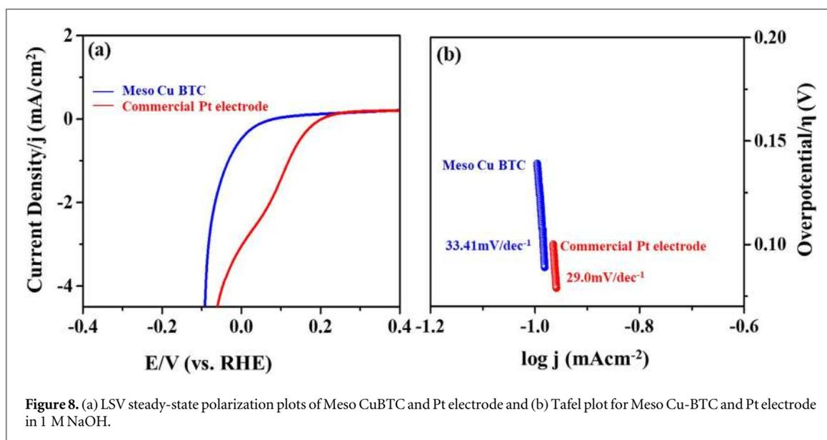
Figure 8. (a) LSV steady-state polarization plots of Meso CuBTC and Pt electrode and (b) Tafel plot for Meso Cu-BTC and Pt electrode in 1 M NaOH.
