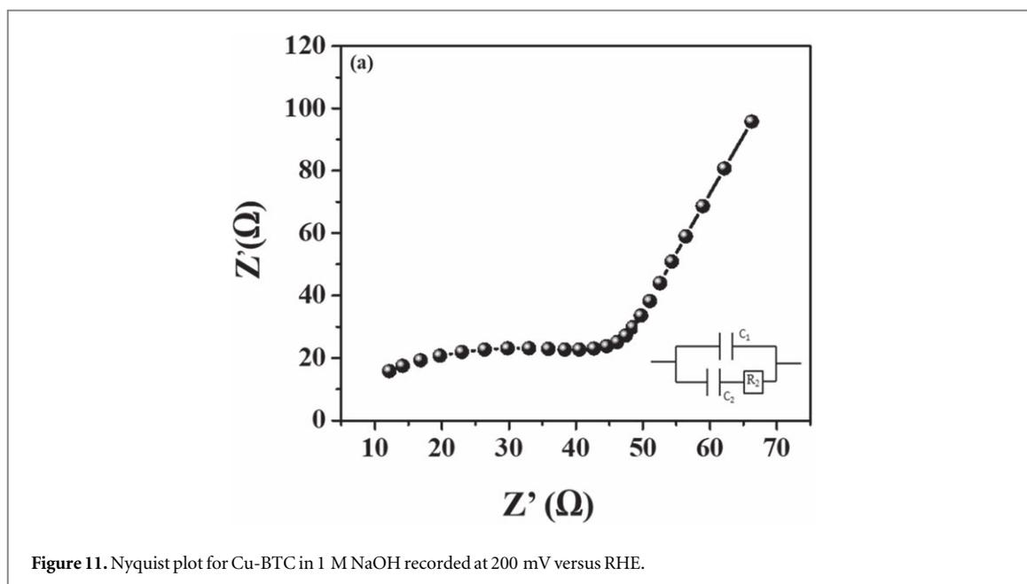
**Figure 11.** Nyquist plot for Cu-BTC in 1 M NaOH recorded at 200 mV versus RHE.
