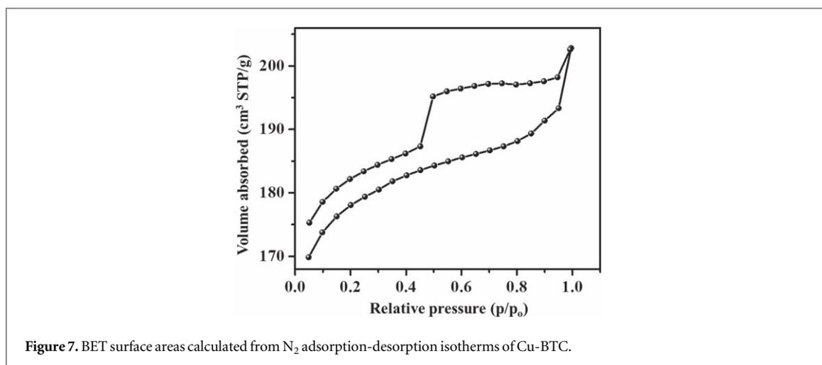
Figure 7. BET surface areas calculated from N<sub>2</sub> adsorption-desorption isotherms of Cu-BTC.
