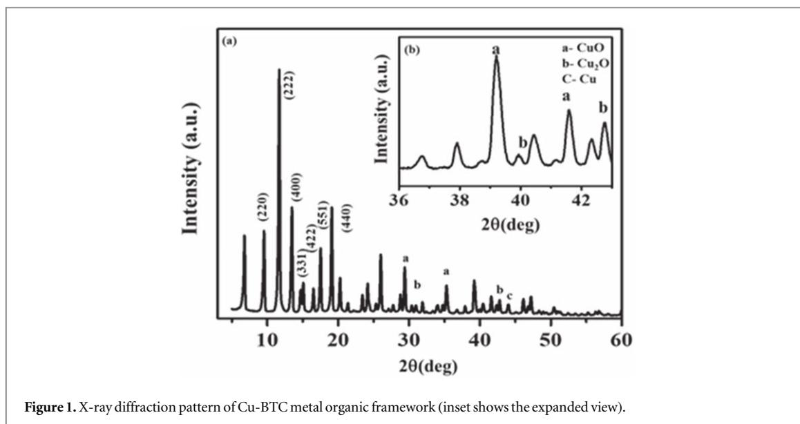
Figure 1. X-ray diffraction pattern of Cu-BTC metal organic framework (inset shows the expanded view).
