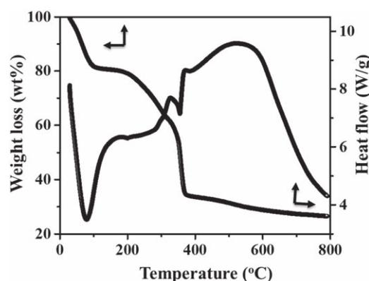
Figure 6. TGA/DSC curves of Cu-BTC Metal organic framework.
