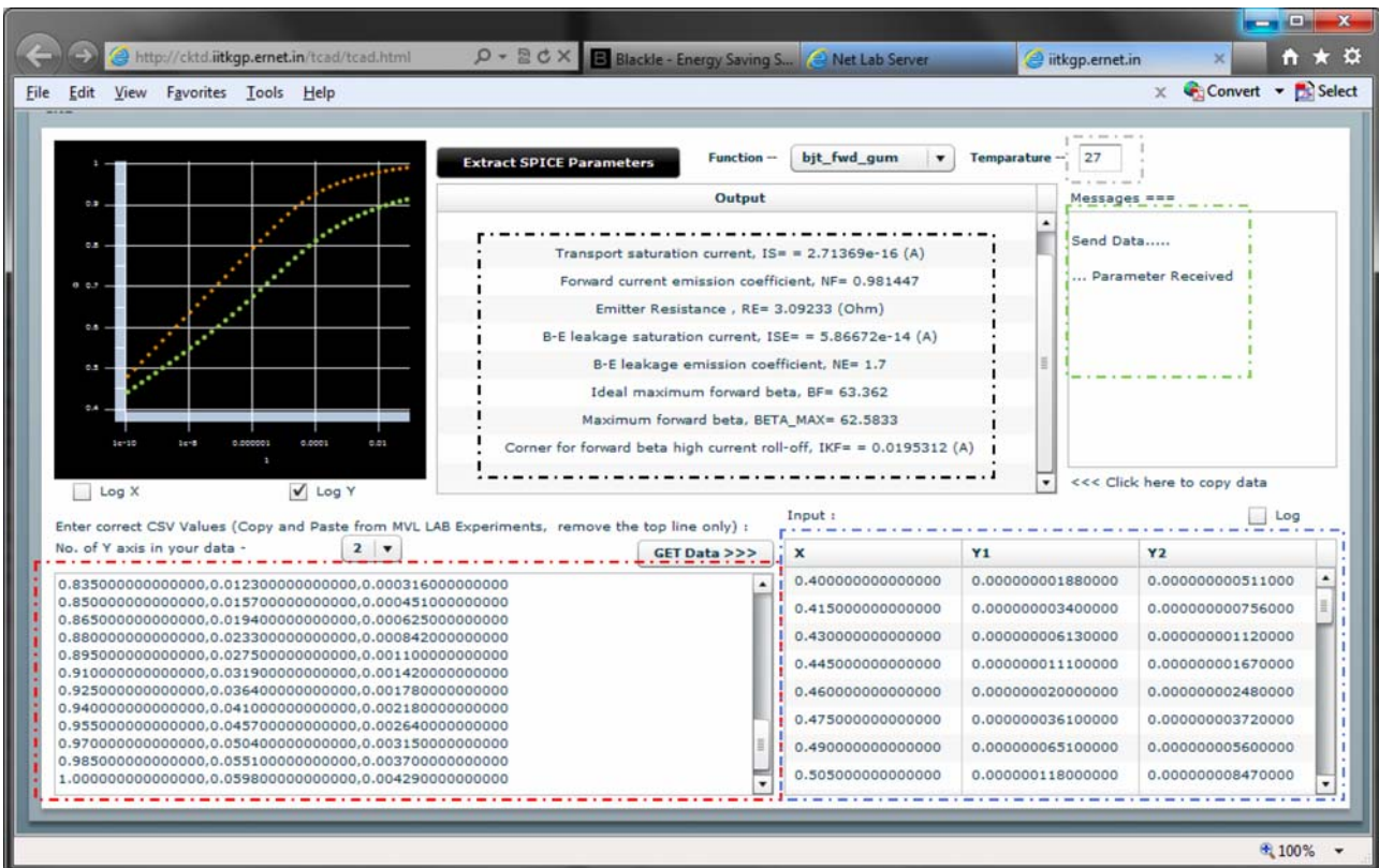
Figure 7. SPICE parameter extraction from Gummel plot. (a) Red enclosure – input data. (b) Blue enclosure – parsed input. (c) Green enclosure – Messages about the request. (d) Black Enclosure – Output. (e) Grey enclosure – additional parameters along with the inputs data.
