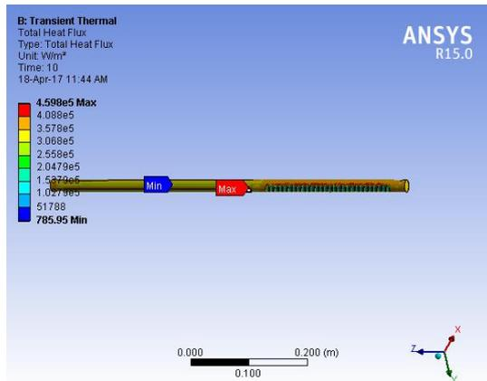
**Figure 4(a).** Heat flux contours for structural steel
