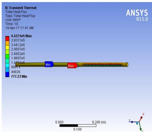
**Figure 3(b).** Heat flux for cast iron
