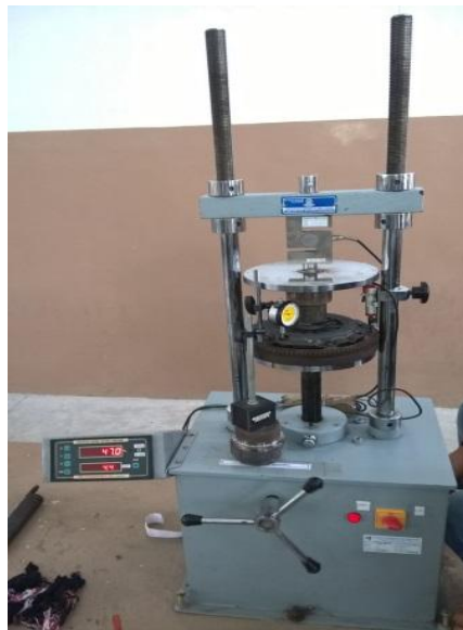
Figure 1. Experimental clutch testing Setup.
