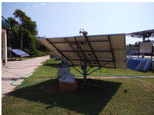
**Figure 8.** Backside of experimental setup with smart tracking system.
