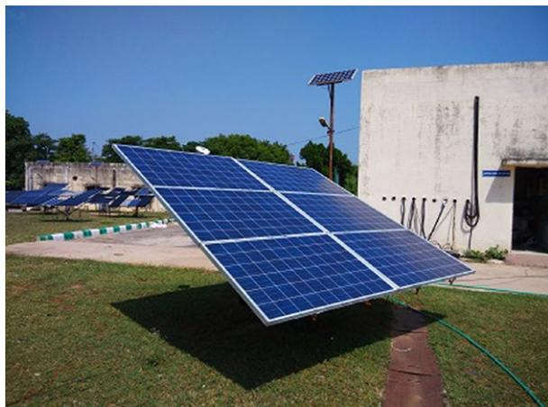
**Figure 7.** Frontside of experimental setup with smart tracking system.
