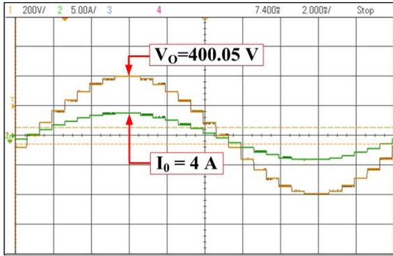
FIGURE 29. 15MLI experimental waveforms with linear load.
