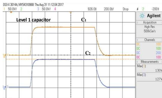
Figure 9. Stage 1 capacitor voltage
