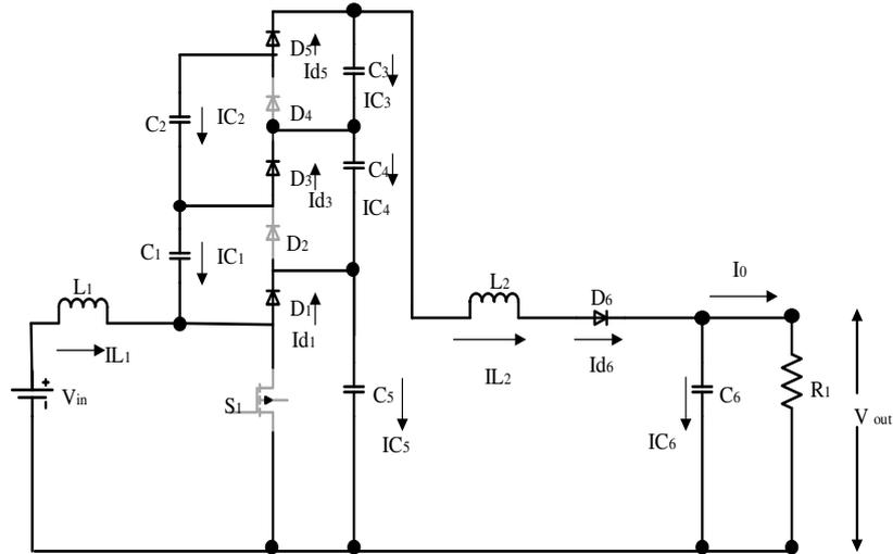
Figure 2. Proposed DC-DC converters turn off mode
