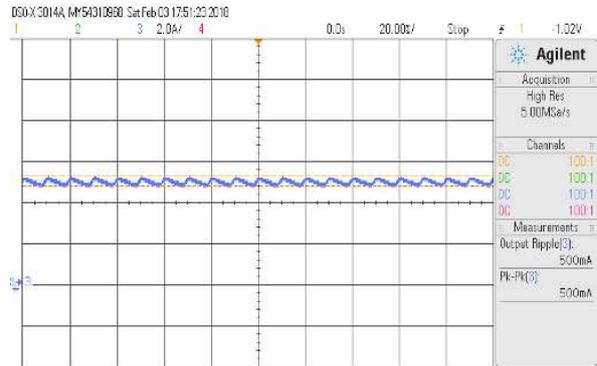
Figure 12. Ripple current waveform of the proposed converter
