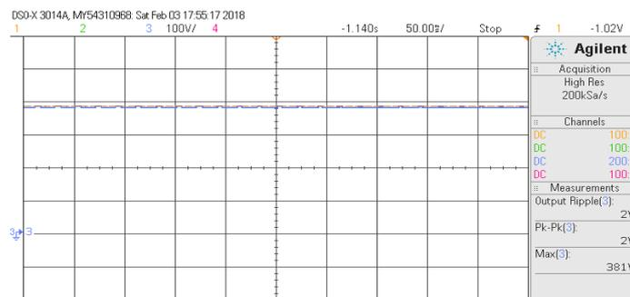
Figure 13. Ripple voltage waveform of the proposed converter
