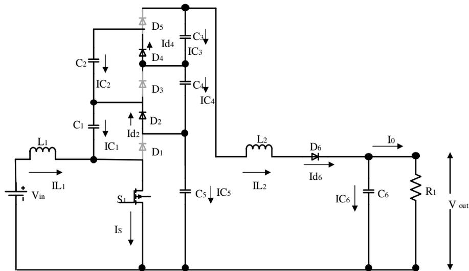
Figure 1. Proposed DC-DC converters turn on mode
