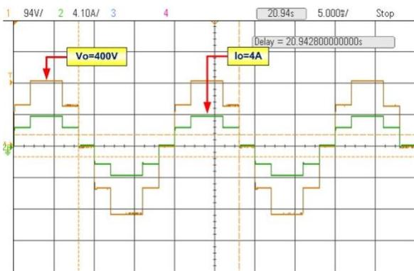
FIGURE 8(b). Experimental output voltage and current waveforms of a five-level inverter
