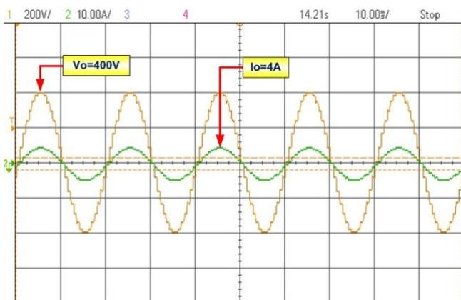
FIGURE 17. Experimental output waveform with R Load
