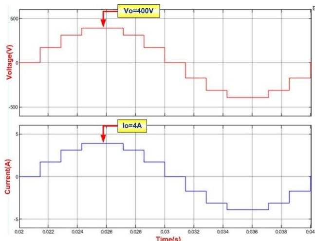
FIGURE 11(a). Simulation output voltage and current waveform of Seven-level inverter
