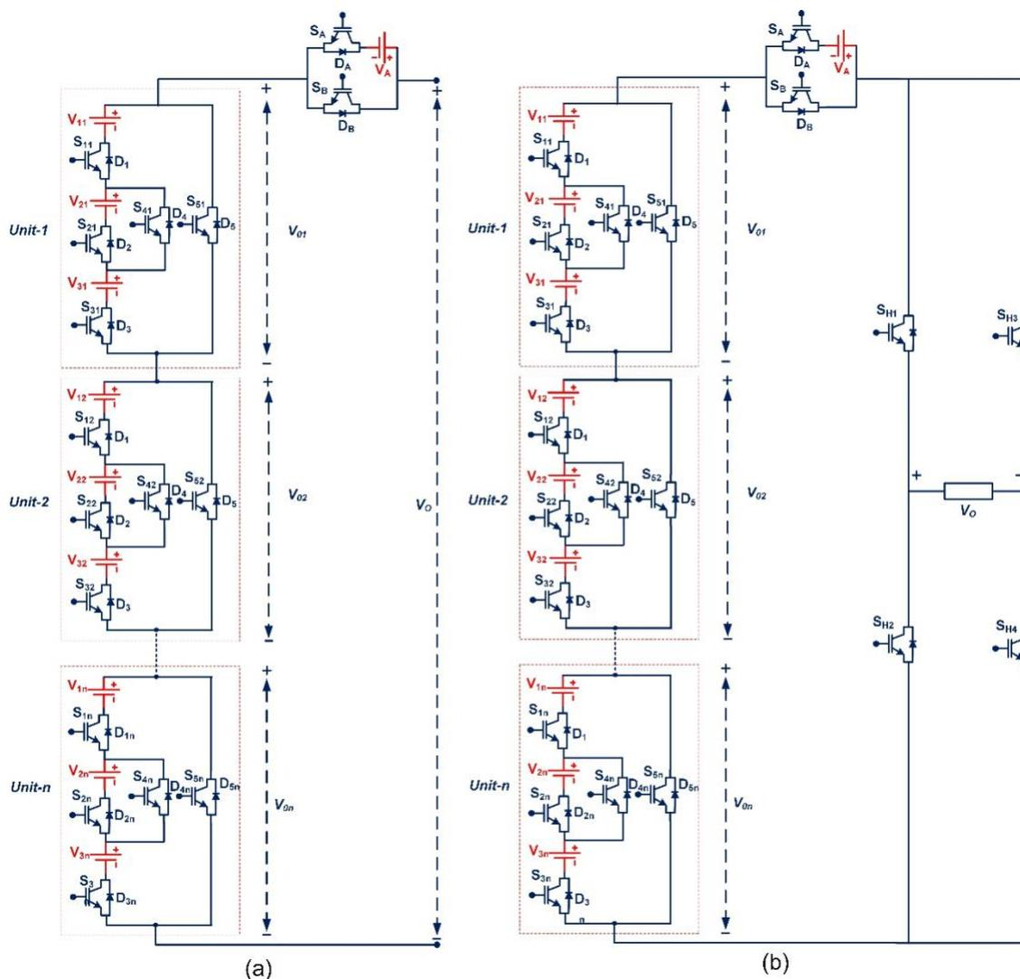
FIGURE 5.1. Developed Cascaded Multilevel Inverter.
