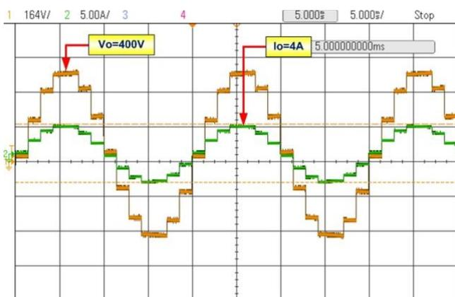
FIGURE 11(b). Experimental output voltage and current waveforms of a seven-level inverter
