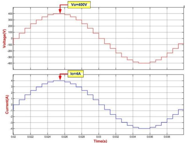
FIGURE 14. Simulation output voltage and current waveforms of a fifteen-level inverter
