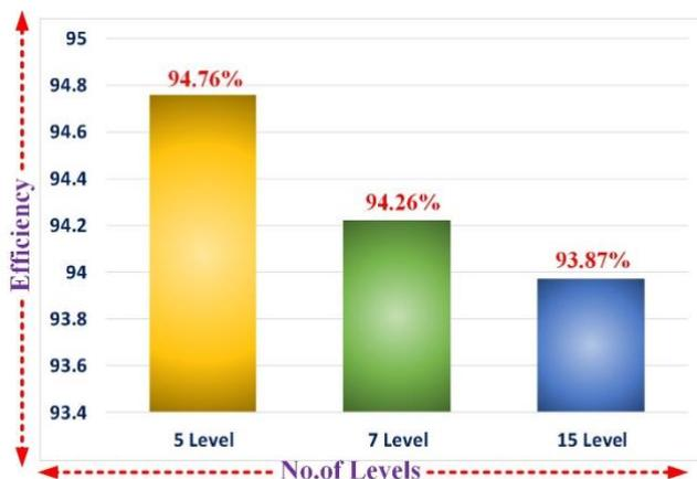
FIGURE 26. Efficiency for various MLI
