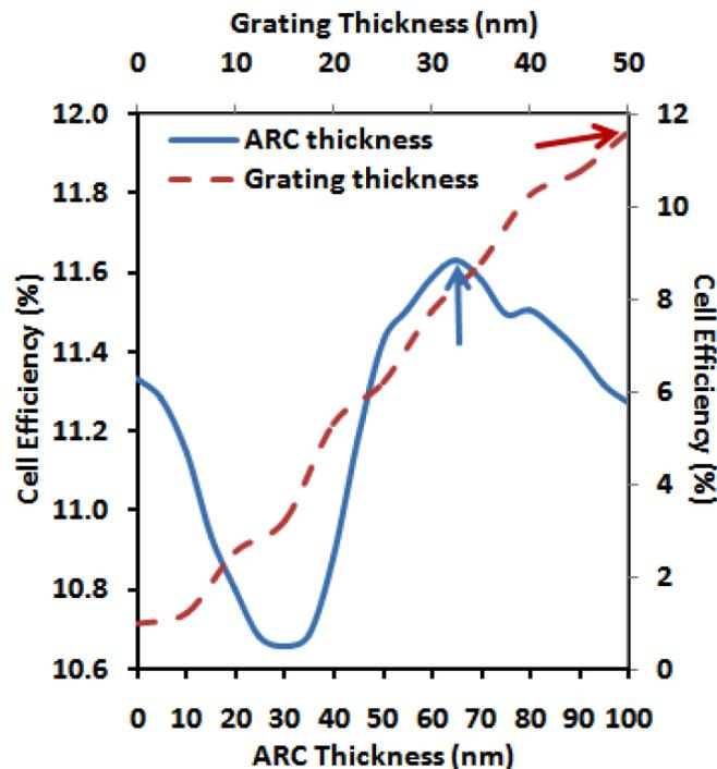
FIG. 2. Solar cell efficiency as a function of ARC thickness (solid line) and grating thickness (dashed line).
