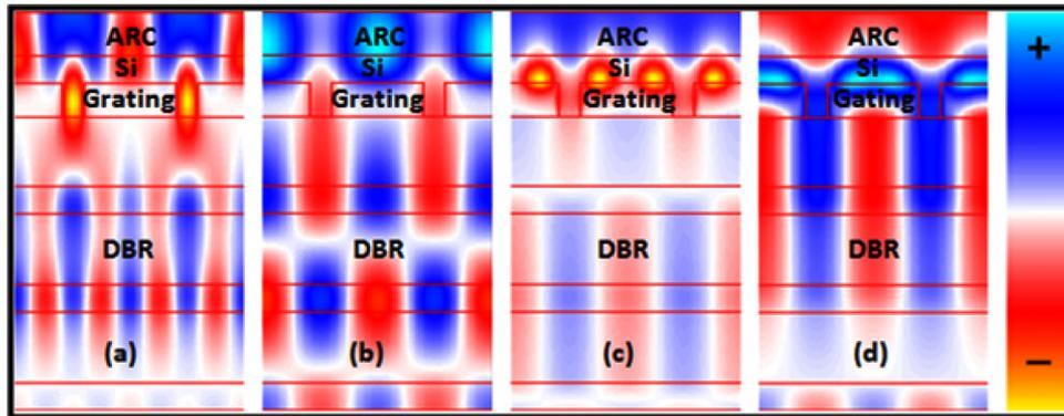
FIG. 7. Electric field profile at 600 & 800 nm (fig.a-b) and magnetic field profile at 741 & 841 nm (fig.c-d).
