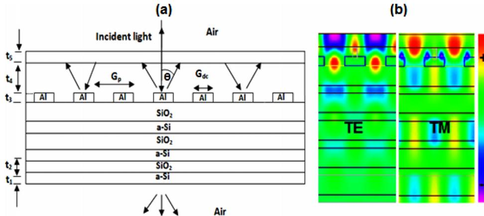
FIG. 1. Schematic diagram of ultrathin silicon solar cell (fig.a) and field distribution in the device for TE and TM polarizations (fig.b).
