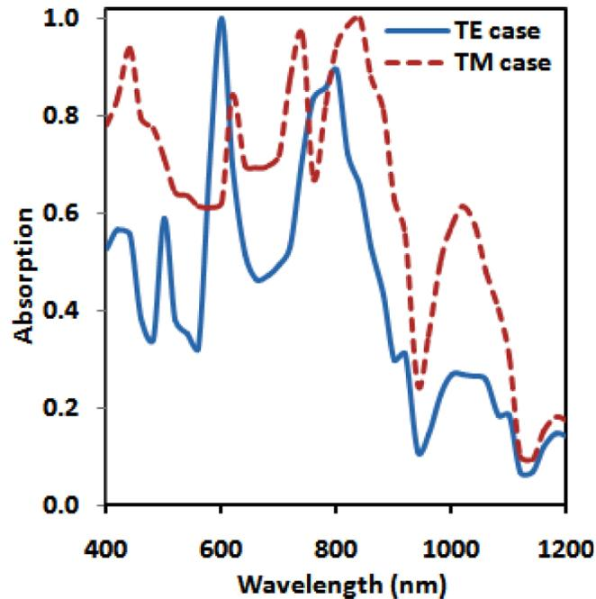
FIG. 6. Light absorption behavior in silicon active layer for TE and TM cases.
