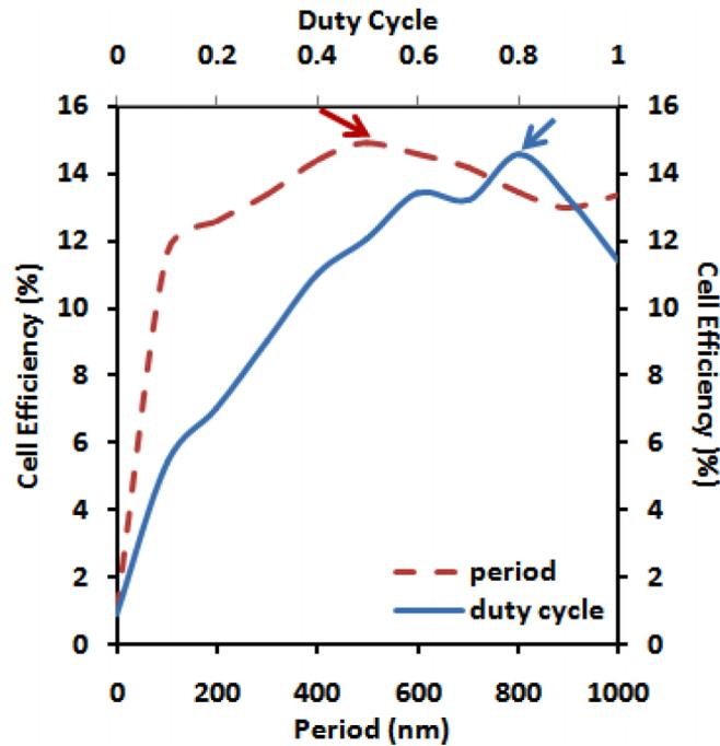
FIG. 4. Solar cell efficiency in accordance with grating duty cycle (solid line) and grating period (dashed line).
