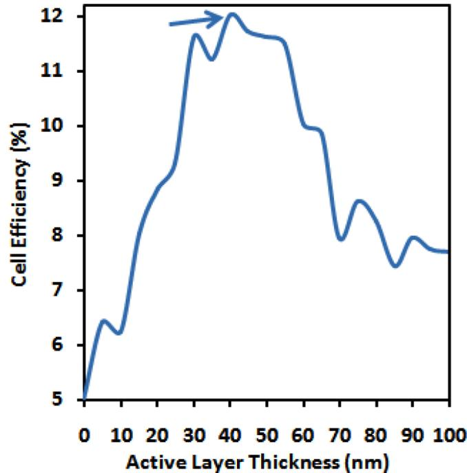
FIG. 3. Solar cell efficiency in accordance with active layer thickness.
