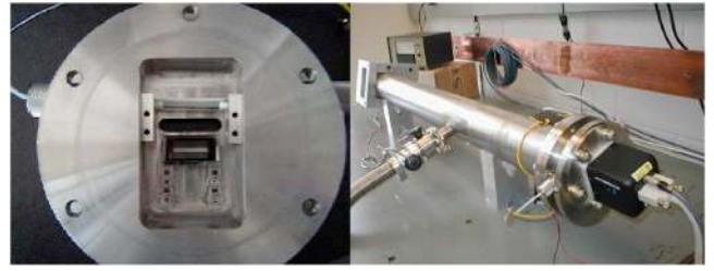
FIG. 3. On the left is the plate, housing the compact fluorescent lamp, the array of slits forming a grating and the 45^\circ mirror. Notice the reflection in the mirror. The grating, which is too fine to be seen, is directly in front of the bulb. The window between the grating and the mirror allows the image to reach the CCD. On the right is the assembled autocollimator. The bellows that connects the autocollimator to the vacuum pump is seen coming from the left. In the foreground is the CCD camera that is connected to a PC for analysis.
