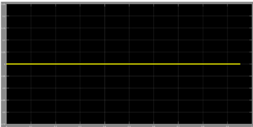
Figure 14. Output (0V) of jammer 1 for input 3. (Legend: x axis = time in 10^{-7} seconds, y axis = voltage in volts).
