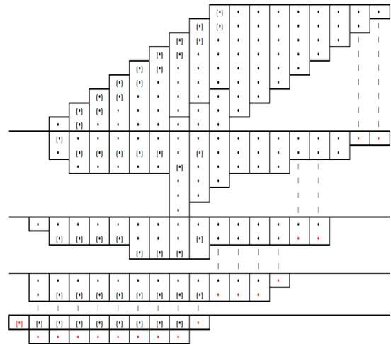
Fig. 4. Dot implementation of Pezaris array multiplier
