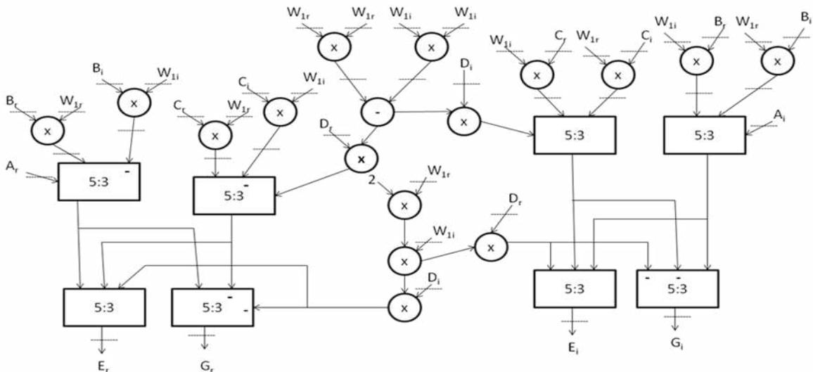
Fig. 6. (a) Butterfly structure using 5 – 3 multicolumn compressor with pipeline (E and G)
