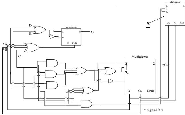
Fig. 3. Implementation of 5-3 compressor with two sign bits
