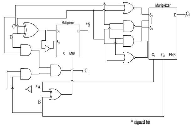
Fig. 2. Implementation of 4-3 compressor with one sign bit
