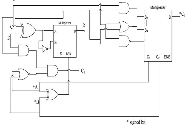
Fig. 1. Implementation of 4-3 compressor with two sign bits
