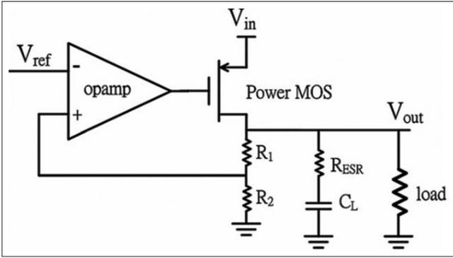
Fig. 1: Basic low dropout schematic
