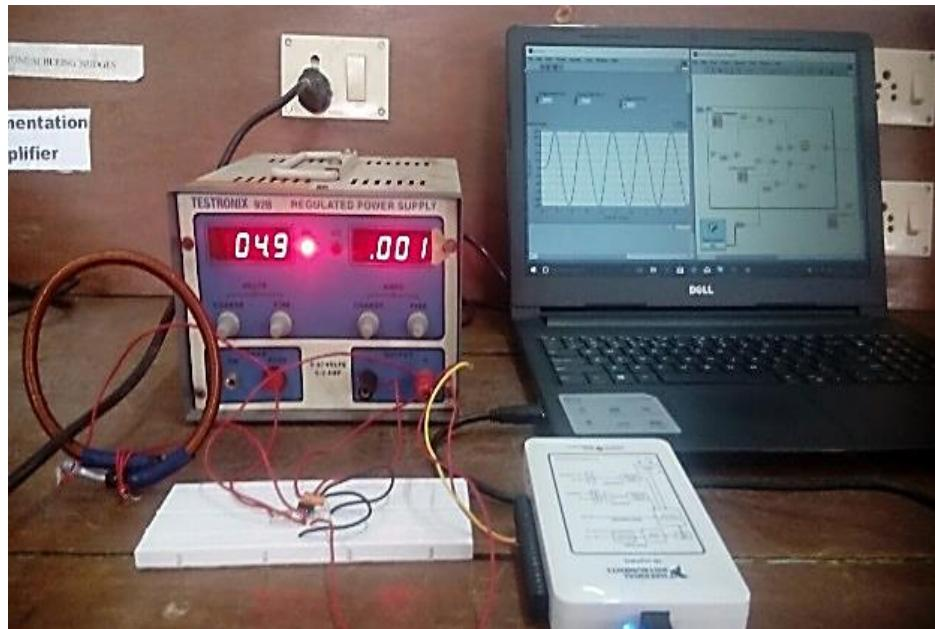
Fig. 2: Hardware Setup of Rogowsk Coil.
