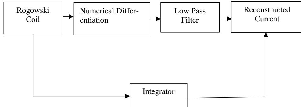
Fig. 1: Block Diagram Representation of Reconstruction Methods.
