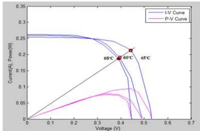
Fig. 3: Output I-V curve under varying temperature
