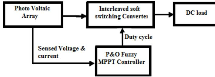
Fig. 1: MPPT controlled PV system block diagram
