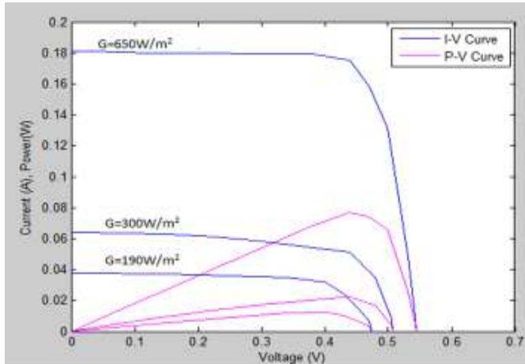
Fig. 4: Output I-V curve under varying illumination
