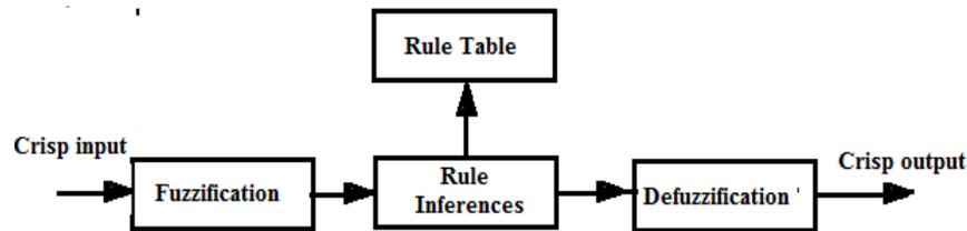
Fig. 9: Block diagram of FLC
