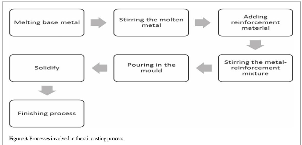
After this step, the molten metal is cast, and then proper machining is done for the desired shape and dimension [21]. It was observed that the composite with 10% weight of alumina is showing better wear resistance. N Bala *et al* has found that to avoid melting of magnesium after preheating, SF<sub>6</sub> along with Argon gases, is added during the stir casting process [22].
