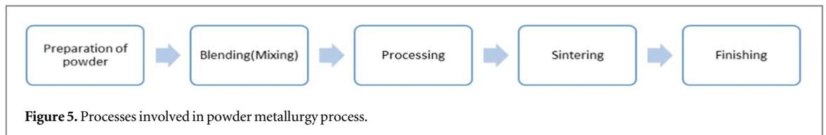
Figure 5. Processes involved in powder metallurgy process.
