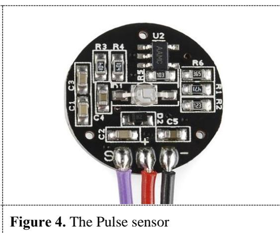
**Figure 4.** The Pulse sensor
