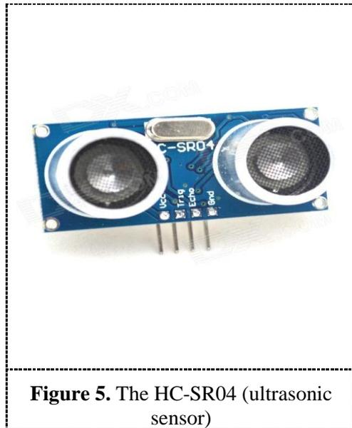
**Figure 5.** The HC-SR04 (ultrasonic sensor)
