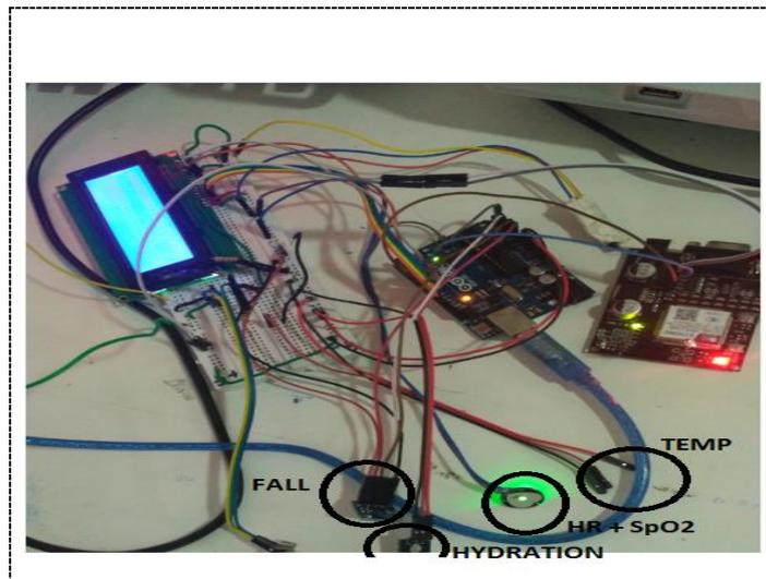
**Figure 7.** Hardware connection for sensors and GSM and Arduino.
