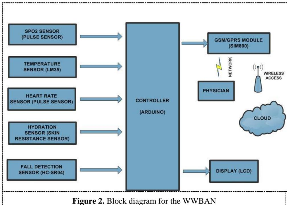
**Figure 2.** Block diagram for the WWBAN
