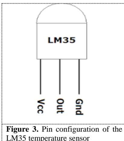
**Figure 3.** Pin configuration of the LM35 temperature sensor
