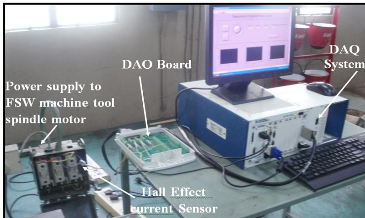
Fig. 2. Hall Effect current sensor and data acquisition system
