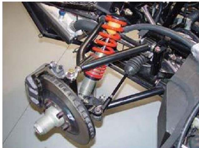
Fig.1-Top left upper view of Double A-Arm suspension
