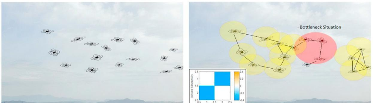
Figure 1: (a) Snapshot of the experimental multi drone setup using the proposed co-simulated organization of cyber physical network system (b) Bottleneck state of multi drone network where yellow aura represents drones in connection and black lines represent routing links, red aura denote the lost links between drones. Inset is the graph of connectivity strength.
