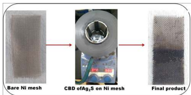
Figure 8. Pictorial representation of \text{Ag}_2\text{S} deposition on Ni mesh via CBD.
