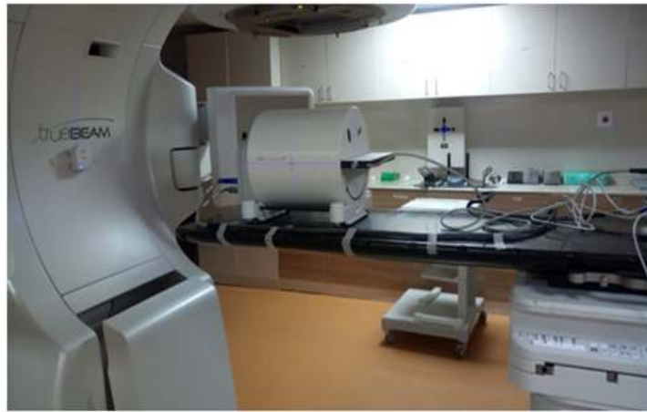
Figure 3: Setup of Octavius 4D Used for Measurement
