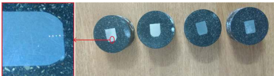
Fig. 12 – Longitudinal cut out specimens for Vickers hardness test.
