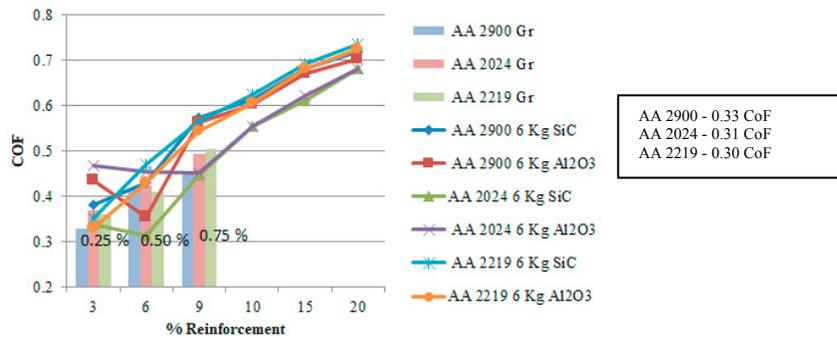
Fig 7: Effect of reinforcement wt% on the coefficient of friction of the composites loaded at 60 N
