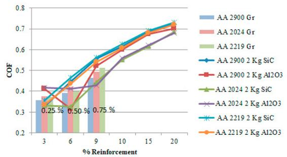
Fig 6: Effect of reinforcement wt% on the coefficient of friction of the composites loaded at 40 N
