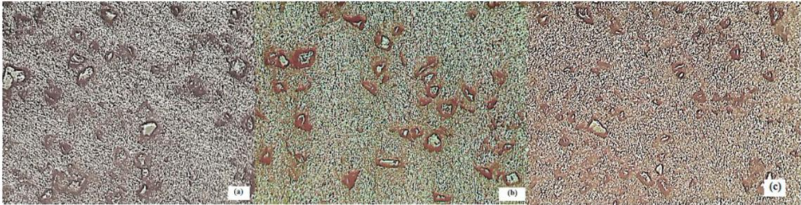
Fig 8: Microstructure of the samples microwave sintered for 6 wt% Al<sub>2</sub>O<sub>3</sub> with (a) AA 2900 and (b) AA 2024 and (c) AA 2219
