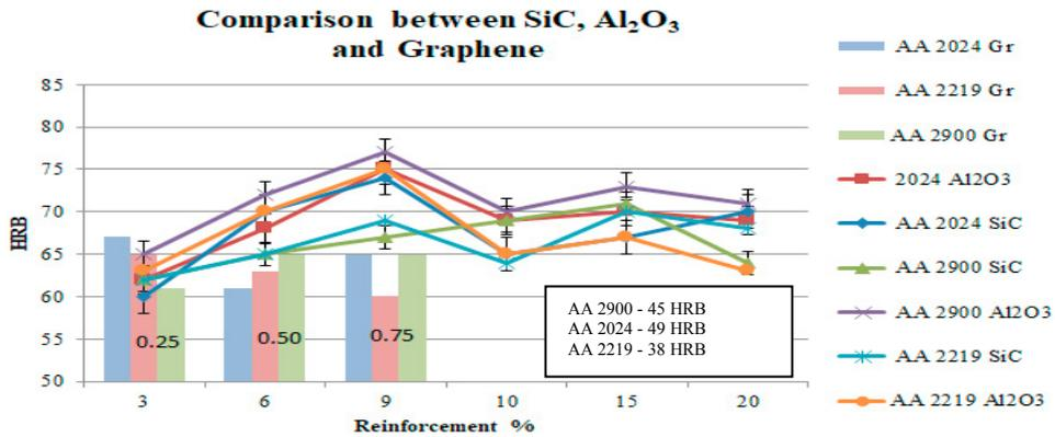
Fig 3: Effect of reinforcement wt% on the Rockwell hardness of the composites
