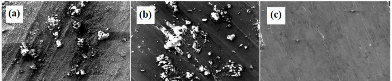
Fig 9: Wear track SEM micrographs (Scale 20 μm) of AA 2900 with 6 wt % Al<sub>2</sub>O<sub>3</sub> at (a) 20 N and (b) 40 N forces and (c) 0.5 wt% Graphene at 40 N
