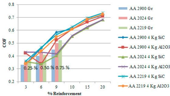
Fig 5: Effect of reinforcement wt% on the coefficient of friction of the composites loaded at 20 N
