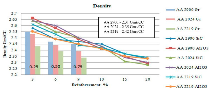
Fig 2: density of aluminium alloy 2900, 2024 and 2219 composites
