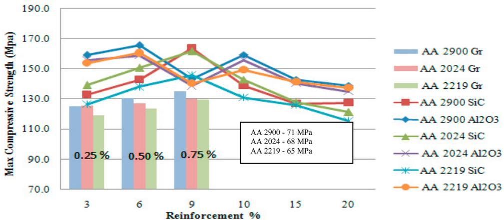
Fig 4: Effect of reinforcement wt% on the Compressive strength of the composites
