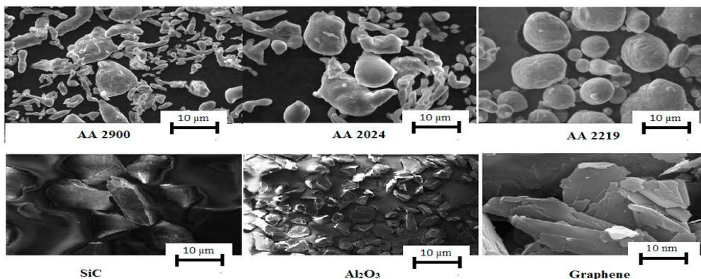
Fig 1: SEM micrographs of Aluminium alloys and reinforcements
