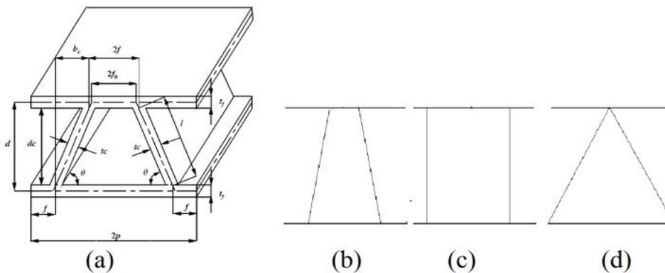
Fig. 1 (a) Dimension of a truss core unit cell [3]. Different topology of truss core sandwich panel, (b) trapezoidal truss core, (c) cellular truss core, and (d) triangular truss core
