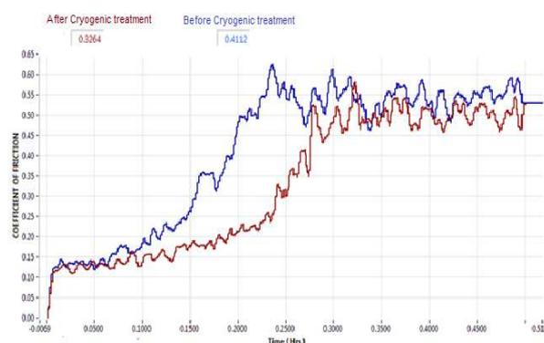
**Fig. 6.** Coefficient of friction versus time plot for additive manufactured 316L SS before and after cryogenic treatment.
