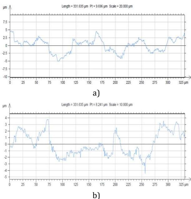
**Fig. 11.** 2D Roughness profile of wear surface in a) untreated & b) cryogenic treated additive manufactured 316L SS sample.
