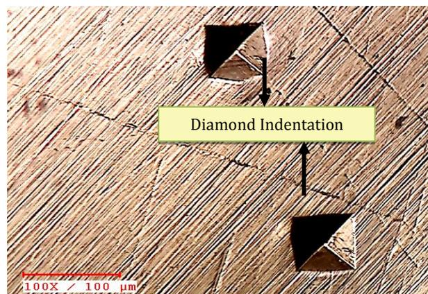
**Fig. 4.** Micro Vickers's diamond indenter indentation on Additive manufactured SS 316 L specimen.
