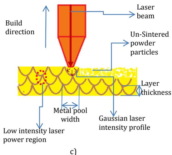
**Fig. 3.** a) Additive manufactured 316L SS microstructure and b) conventional manufactured 316L SS microstructure [32] & c) schematic representation of sintering mechanism in DMLS process.
