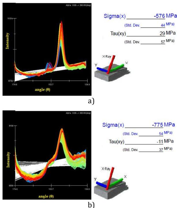
**Fig. 5.** X-ray diffractometer (XRD) pattern and residual stress of the AM 316L SS samples a) before cryogenic treatment and b) after cryogenic treatment.
