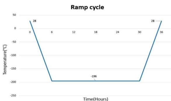
**Fig. 2.** Ramp cycle followed for cryogenic treatment of DMLS part.
