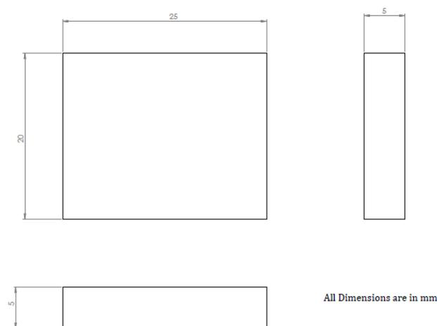
**Fig. 1.** Isometric view of CAD model for specimen fabrication in DMLS.
