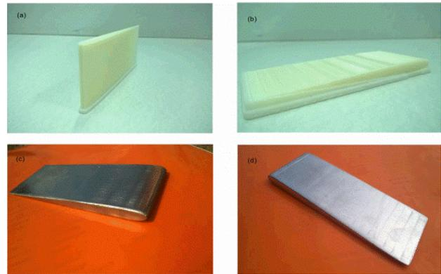
Figure 11. (a) Airfoil with  $90^\circ$  surface angles (b) Airfoil with varying surface angle (c) Electroplated airfoil with  $90^\circ$  surface angles (d) Electroplated airfoil with varying surface angle.
