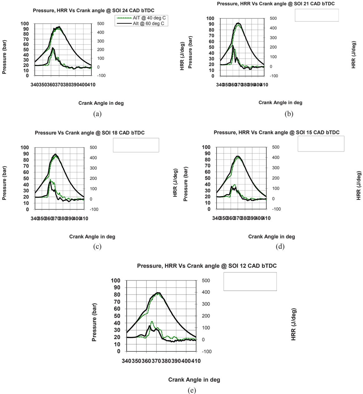
Fig.3 (a), (b), (c), (d), (e) In-cylinder pressure and heat release rate at different SOI and AIT
