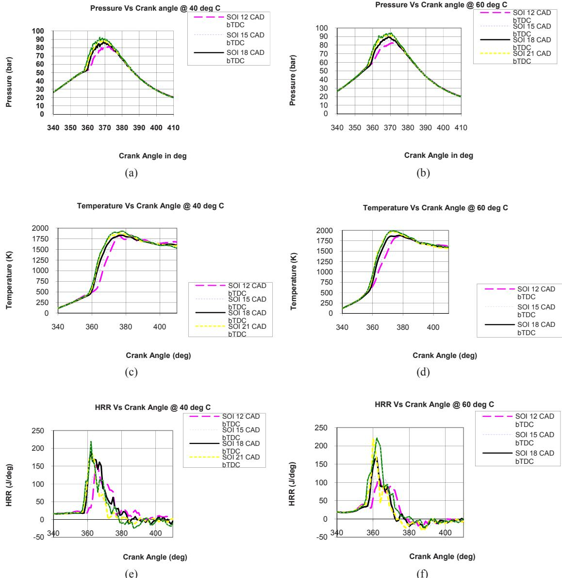
Fig.2 (a) In-cylinder pressure at 40°C of air intake temperature, (b) In-cylinder pressure at 60°C of air intake temperature, (c) Combustion temperature at 40°C of air intake temperature, (d) Combustion temperature at 60°C of air intake temperature, (e) HRR at 40°C of air intake temperature, (f) HRR at 60°C of air intake temperature.
