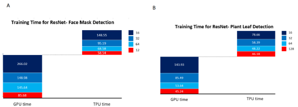
Figure 16 ResNet training time. (A) Training time for ResNet face mask detection. (B) Training time for ResNet plant leaf detection.
