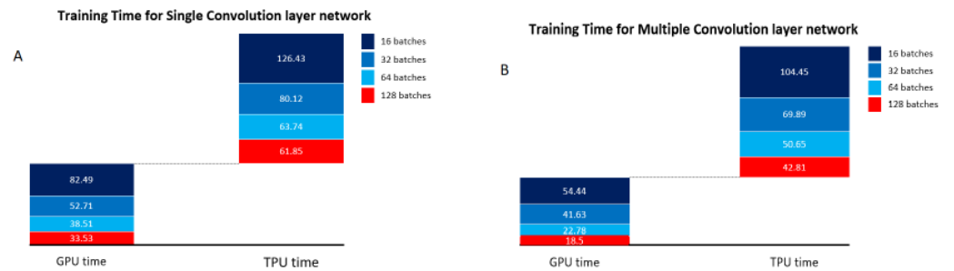
Figure 11 Training time for single and multiple convolutional layer network. (A) Training time for single convolutional layer network. (B) Training time for multiple convolutional layer network.
