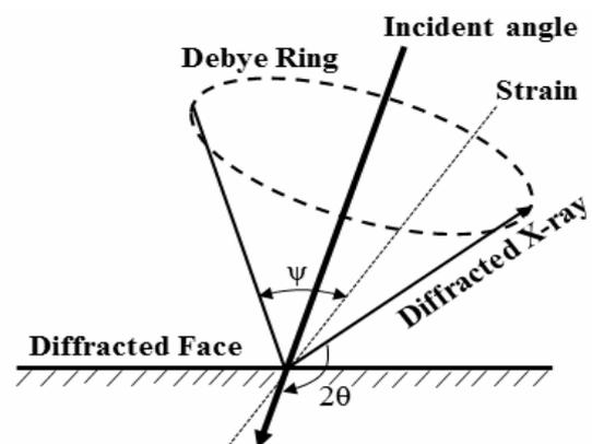
Figure 3. Geometric representation of Debye ring capture
