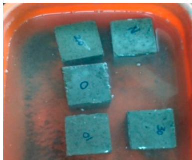
Figure 6. SCC specimens with HIPS in water tank.
