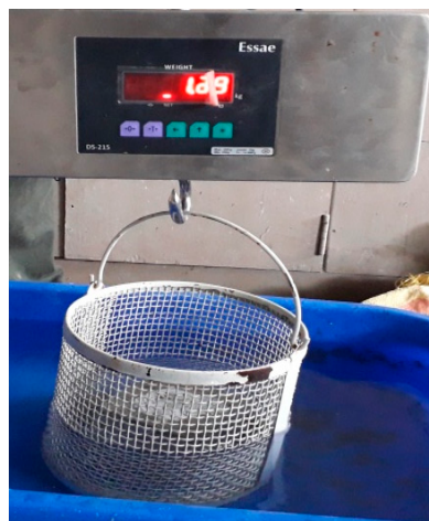
Figure 5. Determination of apparent density for porosity test.
