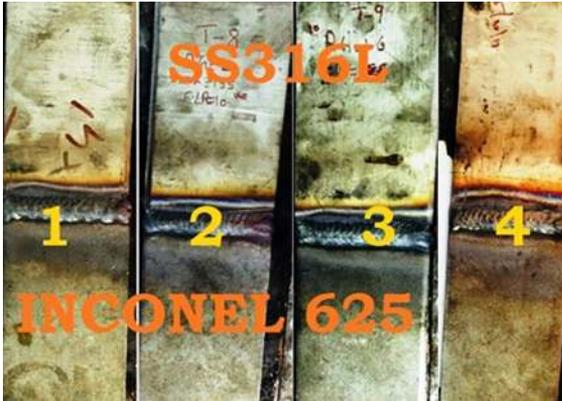
Figure 2. GTA Welded samples
