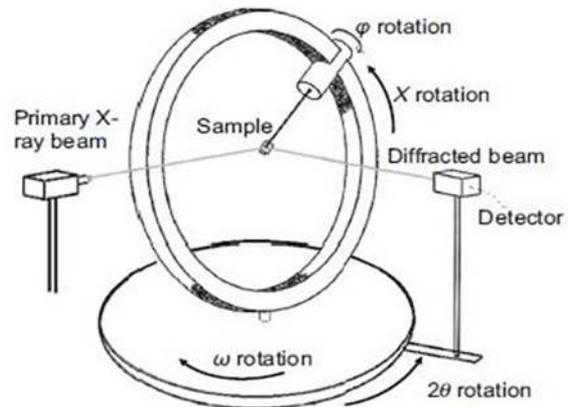
Figure 4. Schematic of goniometer head with detector
