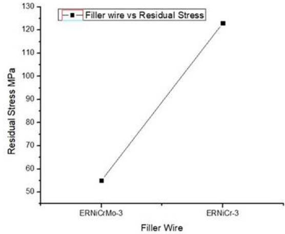
**Figure 10.** Effect of Filler wire on residual stress
