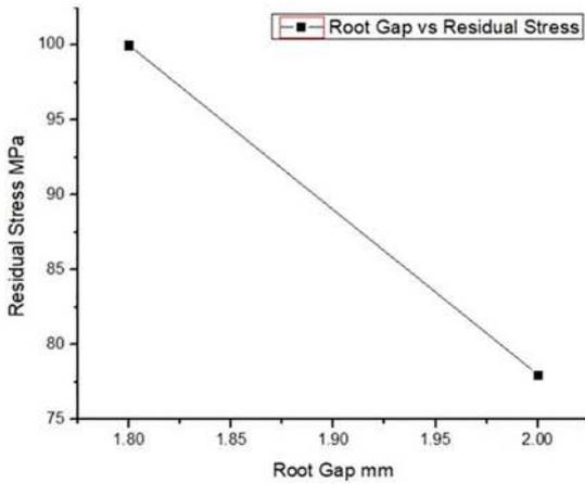
**Figure 8.** Effect of root gap on residual stress
