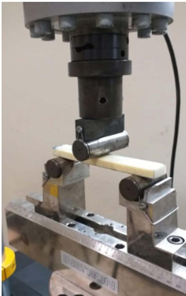
Figure 3. Bending test Instron machine.
