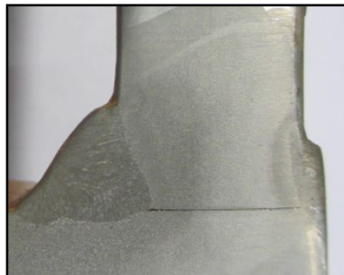
Fig.2. A good penetrations into the root and also a good sidewall fusion
