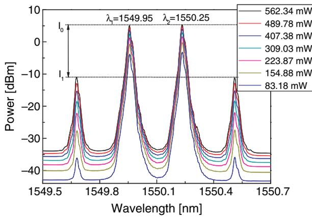
**Fig. 6.** The cw-SPM spectrum of the Si-NCs doped DSF with input pumping power.
