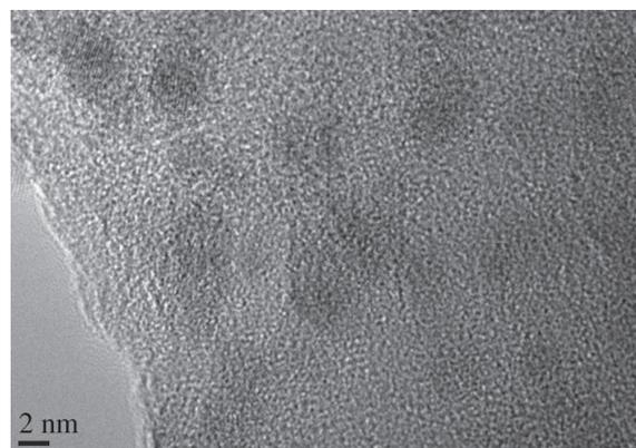
**Fig. 4.** The TEM photograph of the Si-NCs doped DSF preform.
