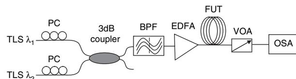
**Fig. 2.** The cw-SPM measurement setup to obtain non-resonant optical nonlinearity: TLS = tunable laser source, PC = polarization controller, BPF = band-pass filter, EDFA = erbium-doped fiber amplifier, FUT = fiber under test, VOA = variable optical attenuator, OSA = optical spectrum analyzer.
