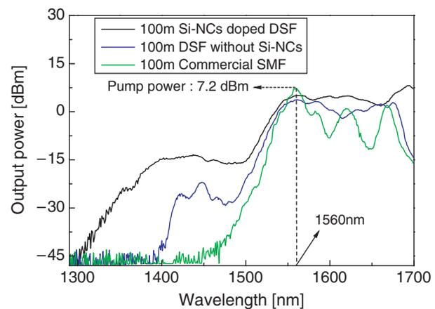
**Fig. 8.** Supercontinuum spectra of the Si-NCs doped DSF, the DSF without Si-NCs, and the commercial SMF upon pumping at 7.2 dBm: the Si-NCs doped DSF (black), the DSF without Si-NCs (blue), and the commercial SMF (green).
