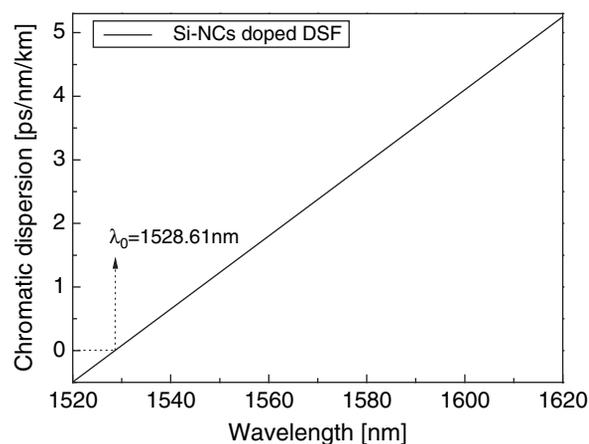
**Fig. 5.** The measured chromatic dispersion of the Si-NCs doped DSF.
