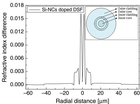
**Fig. 3.** The measured refractive index profile of the Si-NCs doped DSF preform and the schematic cross-section of the Si-NCs doped DSF (the inset).
