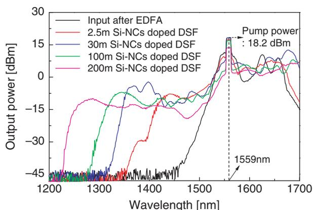
**Fig. 9.** Supercontinuum spectra of the Si-NCs doped DSF with different fiber lengths upon pumping at 18.2 dBm: input after EDFA (black), 2.5 m Si-NCs doped DSF (red), 30 m Si-NCs doped DSF (blue), 100 m Si-NCs doped DSF (green), 200 m Si-NCs doped DSF (pink).
