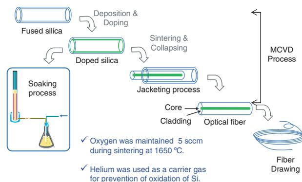
**Fig. 1.** The schematic fabrication steps of the Si-NCs doped DSF: MCVD, doping and drawing processes.
