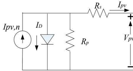
Fig.1. Schematic of One diode model.
