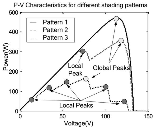
Fig.3. P-V characteristics for shade patterns
