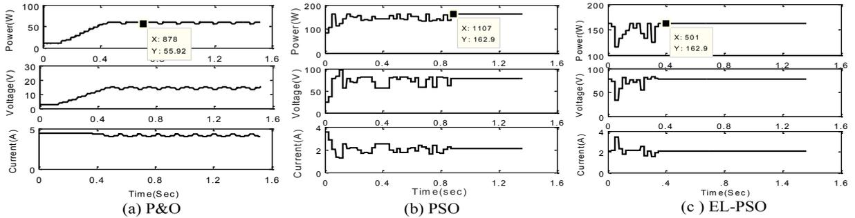
Fig. 4(a). Simulated Results of Power, Voltage and Current waveform for Pattern I.
