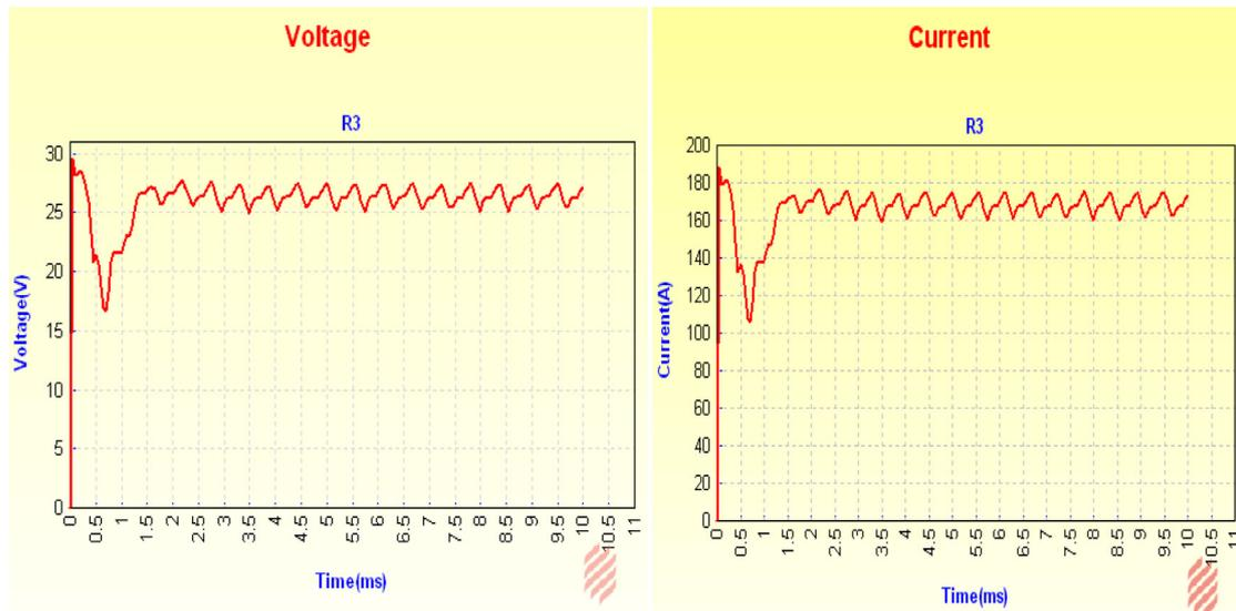
**Figure 5** Load voltage and current in SPA.
