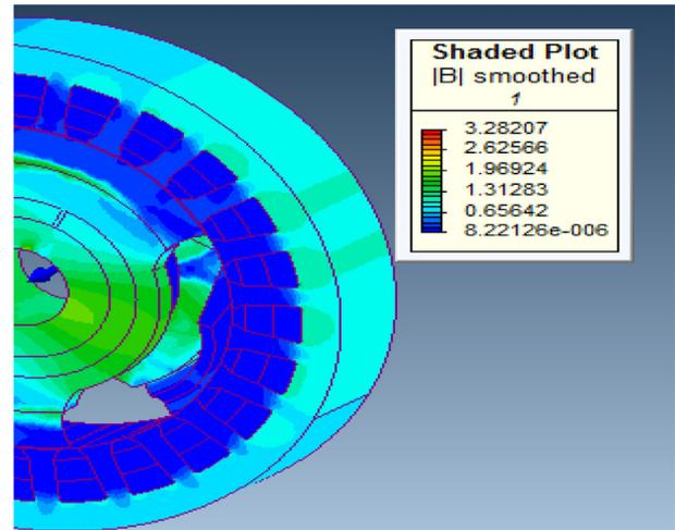
**Figure 7** Flux density plot of CPA.
