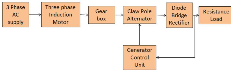
Figure 13 General experimental setup.
