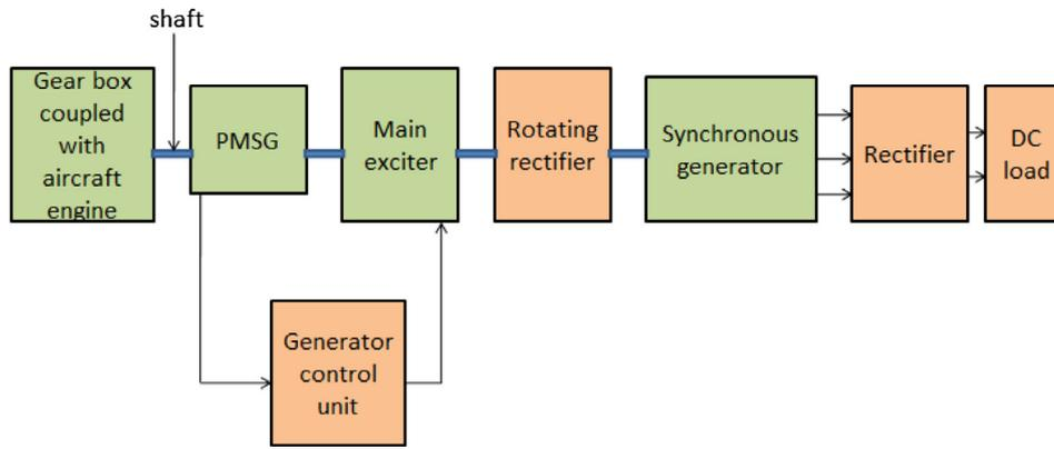
Figure 1 Basic structure of IGS system.
