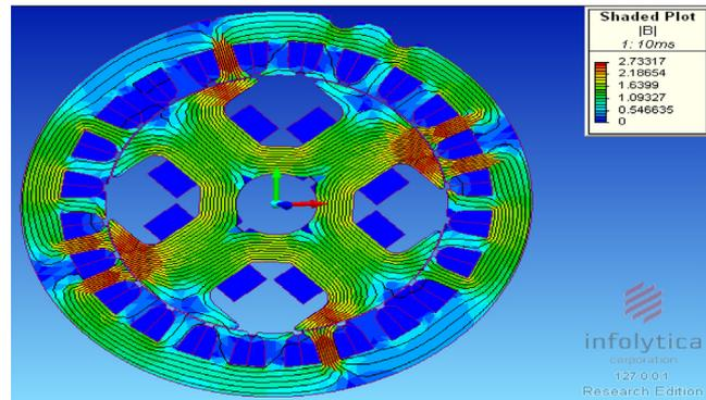
Figure 4 Flux density plot of SPA.
