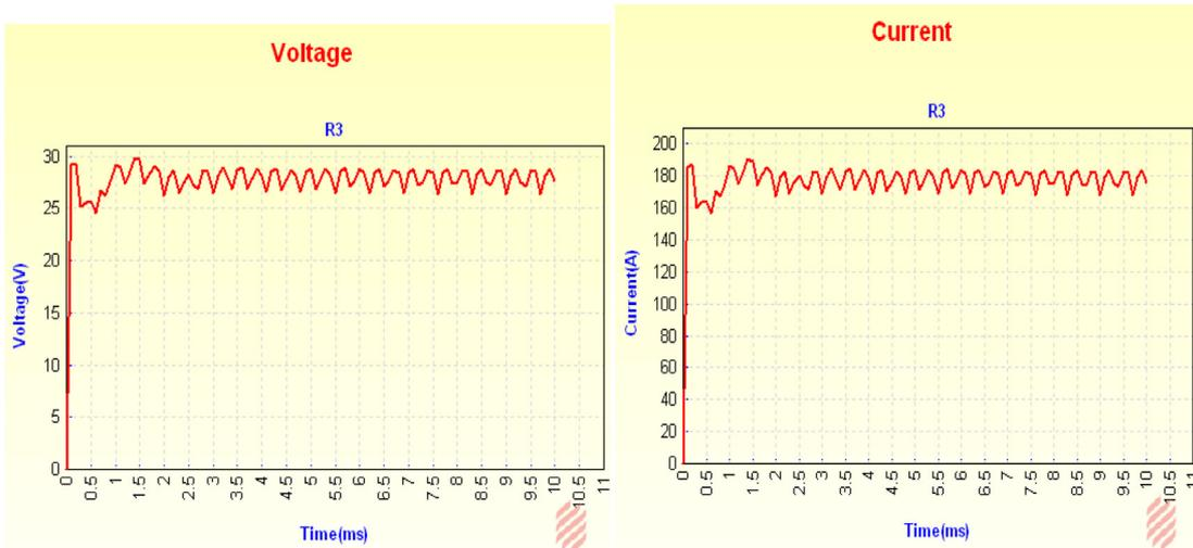
Figure 8 Voltage and current at the load.
