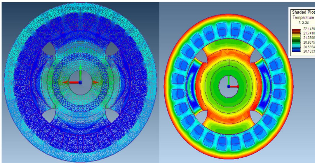
Figure 11 Temperature and heat flow of CPA at 9000 rpm.
