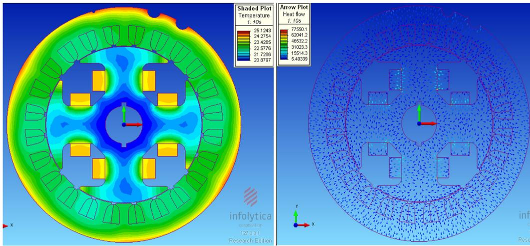
Figure 9 Temperature and heat flow plot of SPA at 9000 rpm.
