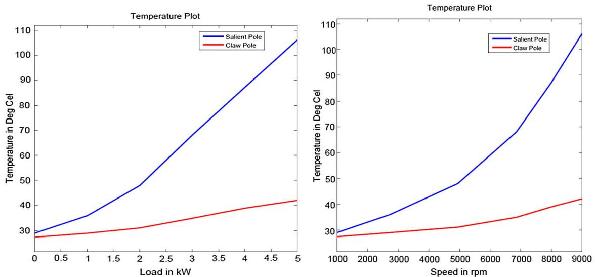
Figure 17 Temperature plot of CPA.
