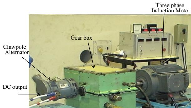
Figure 15 Prototype model of the 5 KW claw pole alternator.
