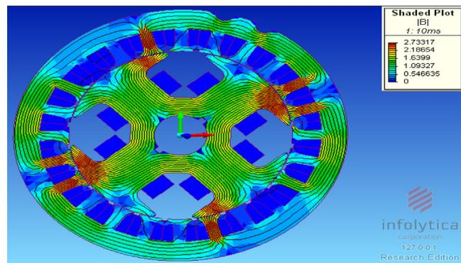
Figure 4 Flux density plot of SPA.
