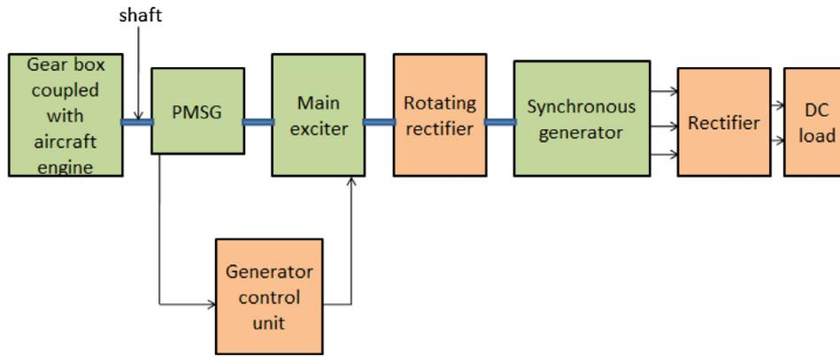
Figure 1 Basic structure of IGS system.
