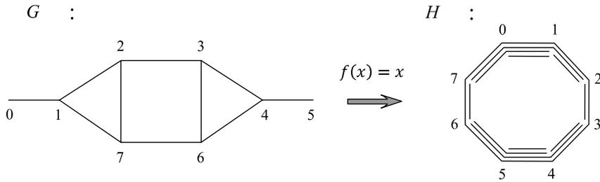
**Fig. 1.** Wiring diagram of a shuffle-exchange network  $G$  into a cycle  $H$  with the edge congestions  $EC_f((0, 1)) = 3, EC_f((1, 2)) = 2, EC_f((2, 3)) = 1, EC_f((3, 4)) = 2, EC_f((4, 5)) = 3, EC_f((5, 6)) = 2, EC_f((6, 7)) = 1$  and  $EC_f((7, 0)) = 2$ .
