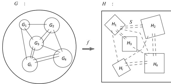
Fig. 3.  $f : G \rightarrow H$  is an embedding and the dotted lines represent edge cut  $S$  in  $H$ .
