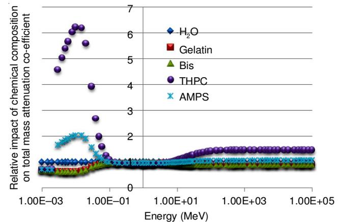
Fig. 7. Impact of chemical composition in energy absorption coefficient
