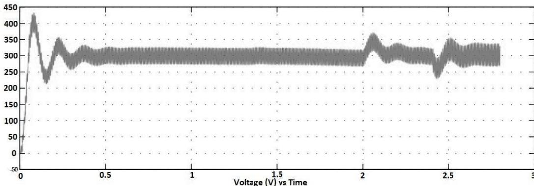
Fig 4. Output voltage of Boost converter
