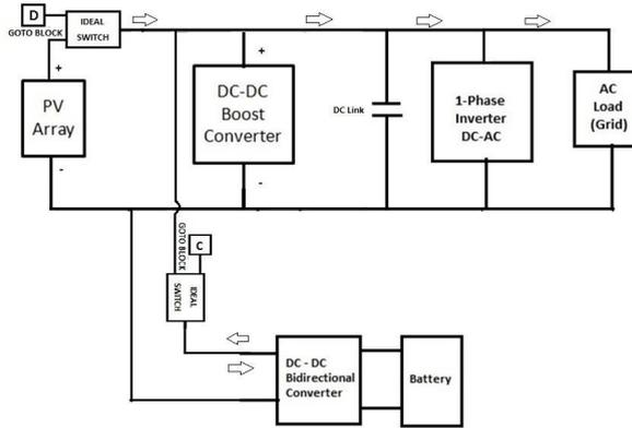
Fig 1. Block Diagram of the proposed system
