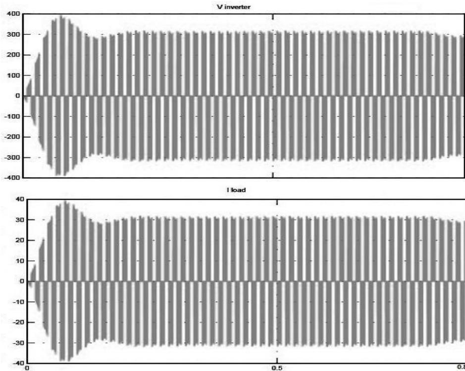
Fig 5. Output voltage and current of load in Mode 1
