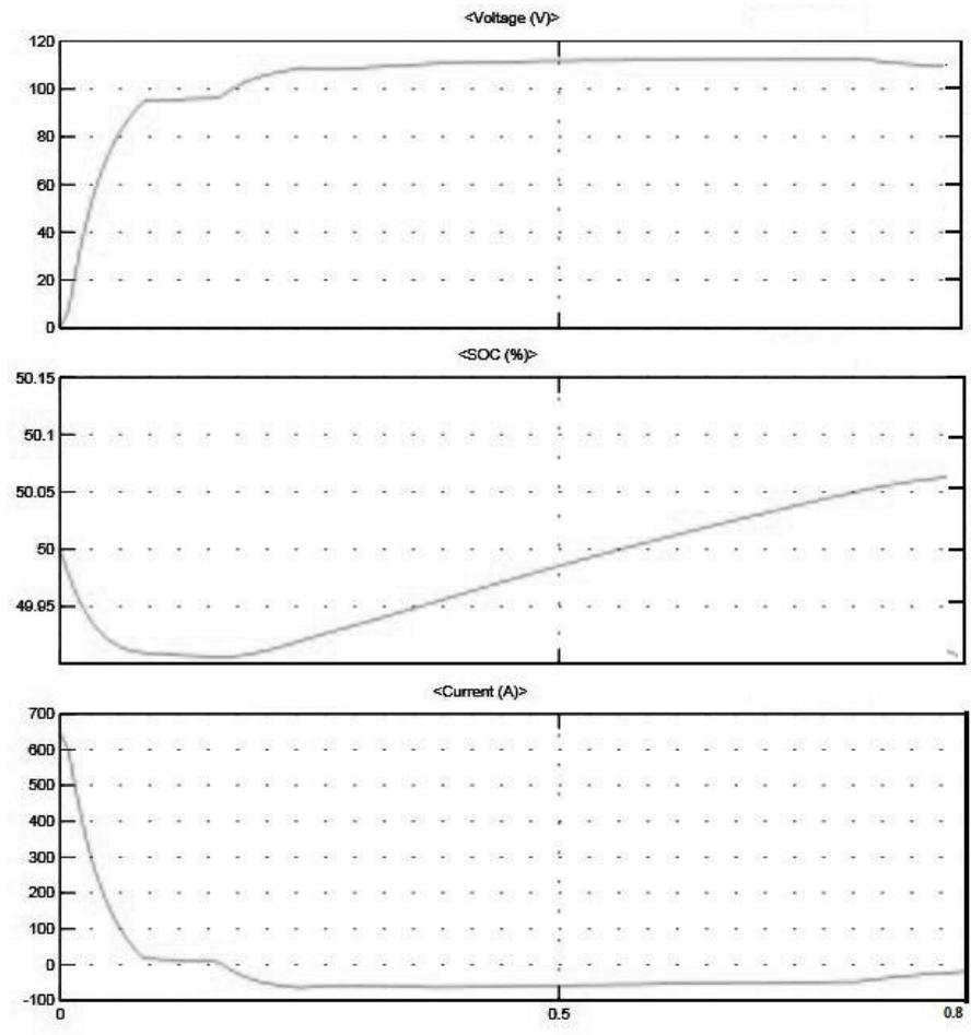
Fig.6. Output Voltage, State of Charge and current graph of battery during mode 1(charging)
