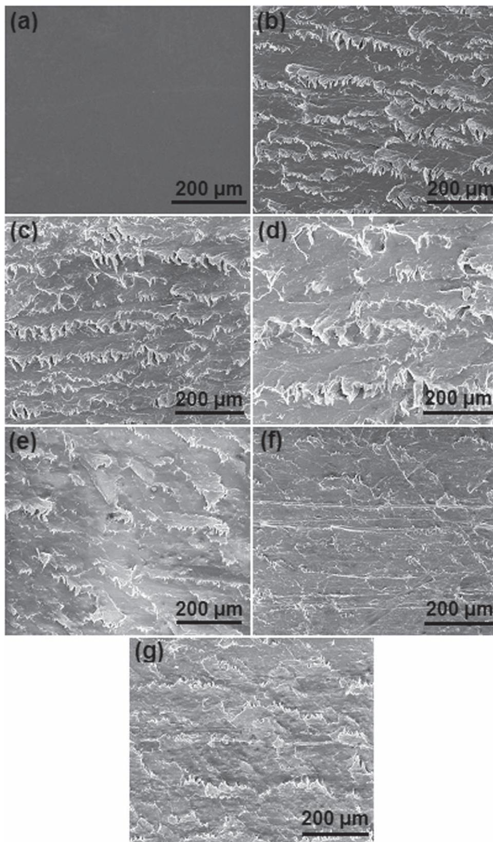
**Figure 10.** SEM images of (a) neat PVA, (b) PVA/NiS nanocomposite films filled with 0.5 wt% NiS NPs, (c) 1.0 wt% NiS NPs, (d) 1.5 wt% NiS NPs, (e) 2.0 wt% NiS NPs, (f) 2.5 wt% NiS NPs and (g) 3.0 wt% NiS NPs.
