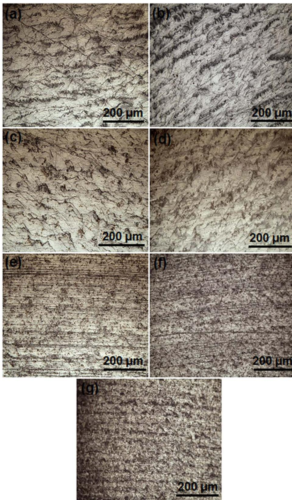
**Figure 7.** POM images of (a) neat PVA, (b) PVA/NiS nanocomposite films loaded with 0.5 wt% NiS NPs, (c) 1.0 wt% NiS NPs, (d) 1.5 wt% NiS NPs, (e) 2.0 wt% NiS NPs, (f) 2.5 wt% NiS NPs and (g) 3.0 wt% NiS NPs.
