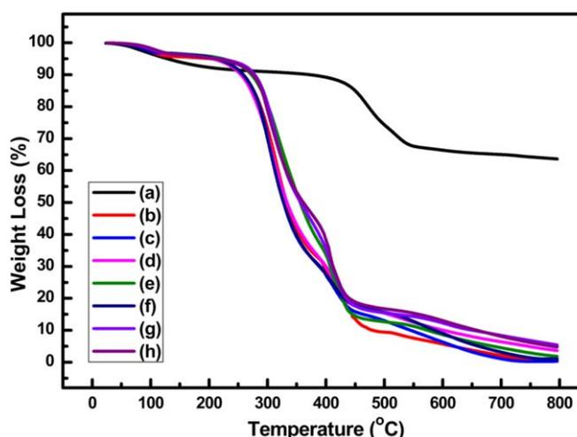
**Figure 5.** TGA plots of (a) NiS NPs, (b) neat PVA, (c) PVA/NiS nanocomposite films embedded with 0.5 wt% NiS NPs, (d) 1.0 wt% NiS NPs, (e) 1.5 wt% NiS NPs, (f) 2.0 wt% NiS NPs, (g) 2.5 wt% NiS NPs and (h) 3.0 wt% NiS NPs.
