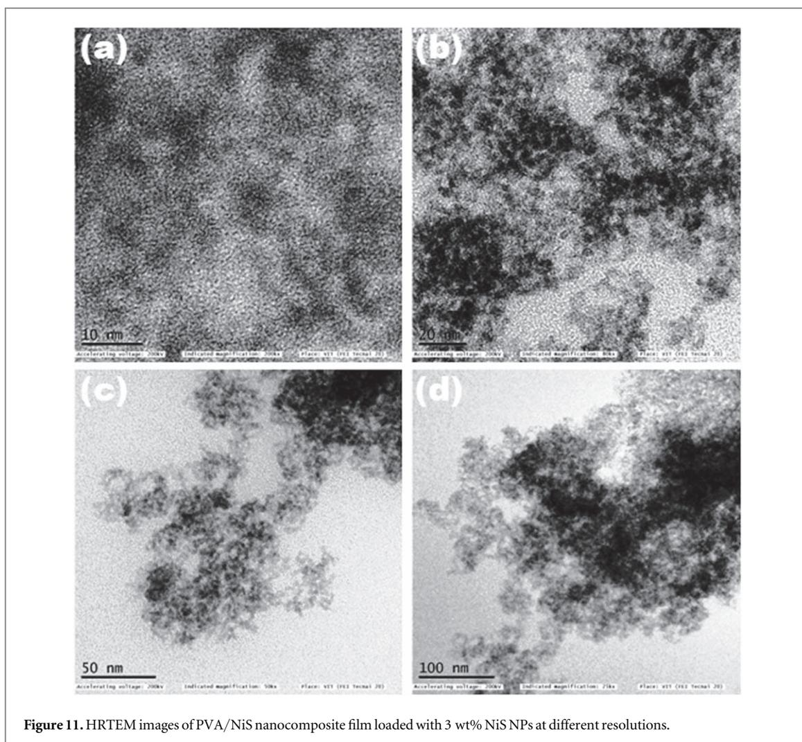
**Figure 11.** HRTEM images of PVA/NiS nanocomposite film loaded with 3 wt% NiS NPs at different resolutions.
