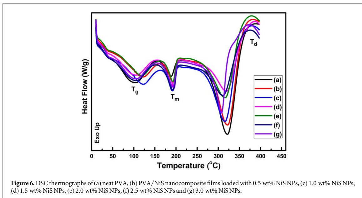
**Figure 6.** DSC thermographs of (a) neat PVA, (b) PVA/NiS nanocomposite films loaded with 0.5 wt% NiS NPs, (c) 1.0 wt% NiS NPs, (d) 1.5 wt% NiS NPs, (e) 2.0 wt% NiS NPs, (f) 2.5 wt% NiS NPs and (g) 3.0 wt% NiS NPs.
