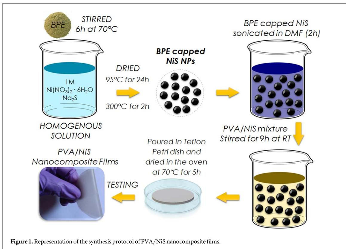
**Figure 1.** Representation of the synthesis protocol of PVA/NiS nanocomposite films.
