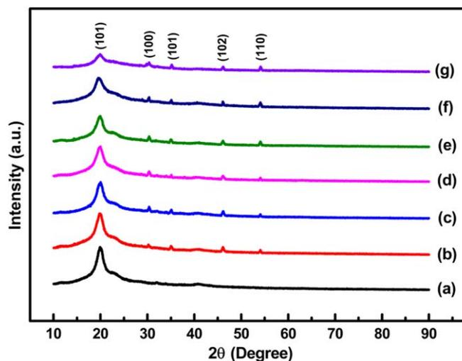
**Figure 4.** XRD patterns of (a) neat PVA, (b) PVA/NiS nanocomposite films filled with 0.5 wt% NiS NPs, (c) 1.0 wt% NiS NPs, (d) 1.5 wt% NiS NPs, (e) 2.0 wt% NiS NPs, (f) 2.5 wt% NiS NPs and (g) 3.0 wt% NiS NPs.
