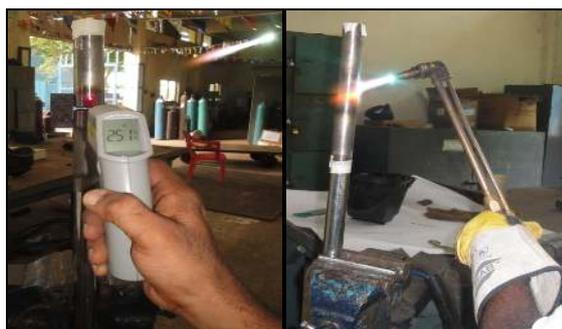
**Figure 1: Pre heating the test specimen**
