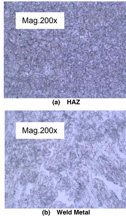
Figure 5: Microstructure of Helium gas specimen HAZ & WM
