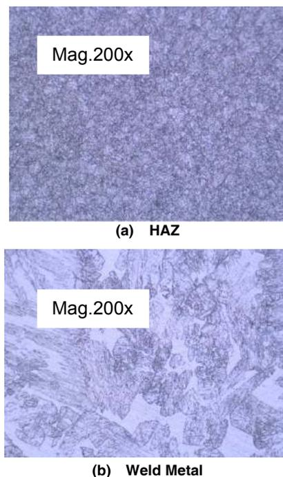
Figure 4: Microstructure of Argon gas specimen HAZ & WM
