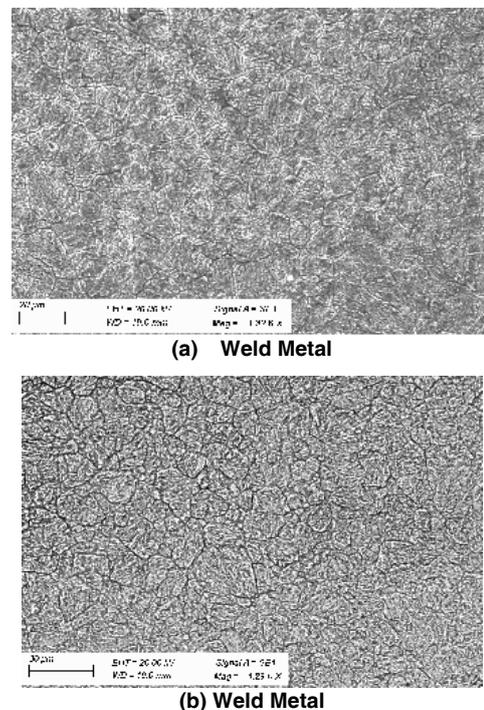
Figure: 9 SEM image Argon 50% & Helium 50% weld Specimen
