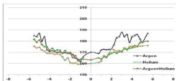
**Figure 2: Micro hardness for different shielding gas**
