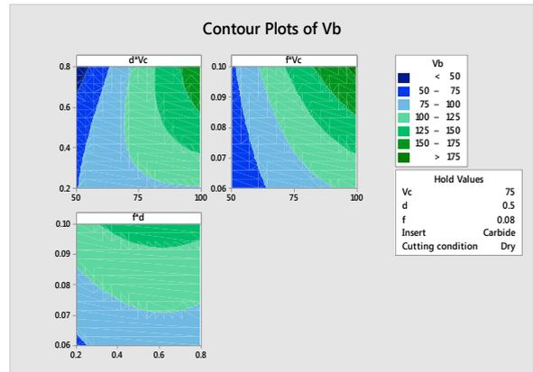
Fig. 8. Contour plot for wear
