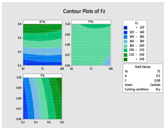
Fig. 2. Contour plot for cutting force
