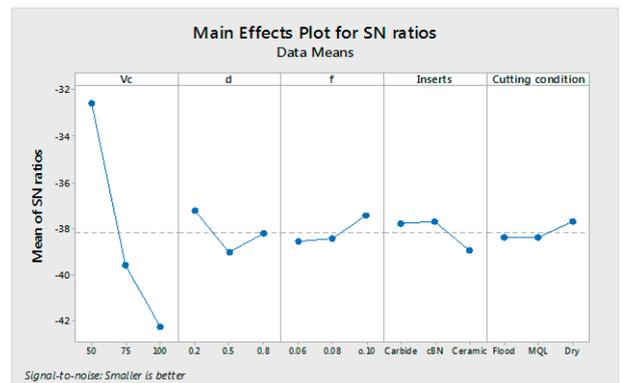
Fig 7 – Signal to noise ratio for flank wear
