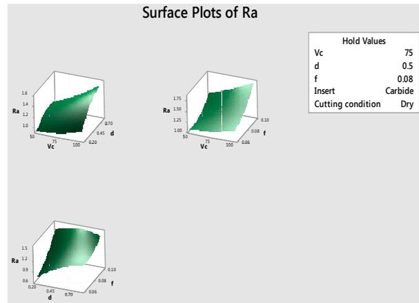
Fig. 6. Surface plot for Ra
