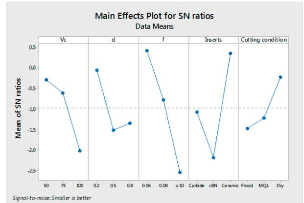
Fig. 4. S/N ratio graph for surface roughness
