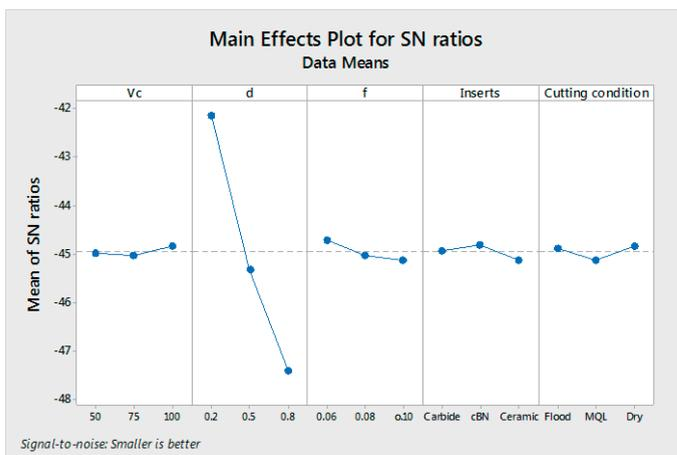
Fig.1. S/N ratio graph for cutting force Fz
