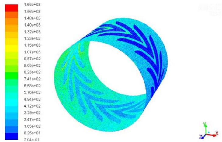
Fig.7 dynamic pressure contour for eccentricity ratio 0.4.
