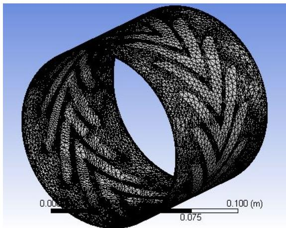
Fig 2: Mesh of the fluid film.
