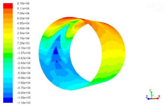
Fig.6 Static pressure contour for eccentricity ratio 0.4.
