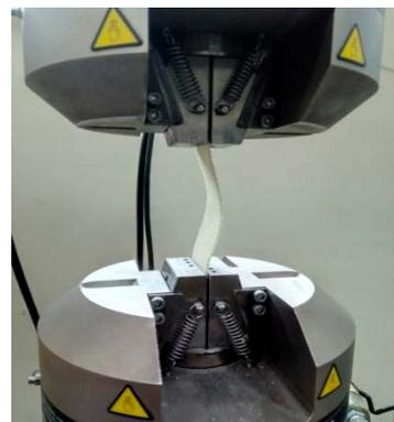
**Figure 7.** Buckling of a composite sample.
