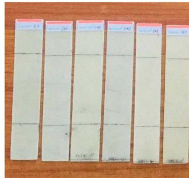
**Figure 6.** Samples of the woven flax/bio epoxy (WFBE) laminated composite.
