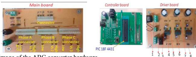
Fig. 9. Image of the ABC converter hardware
