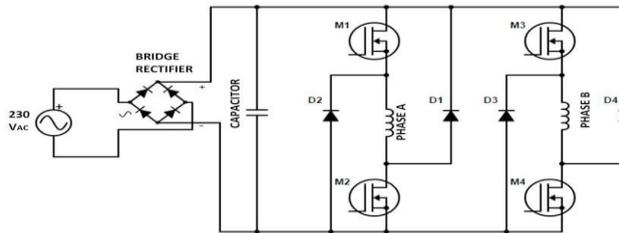
Fig. 7. Asymmetric Bridge Converter
