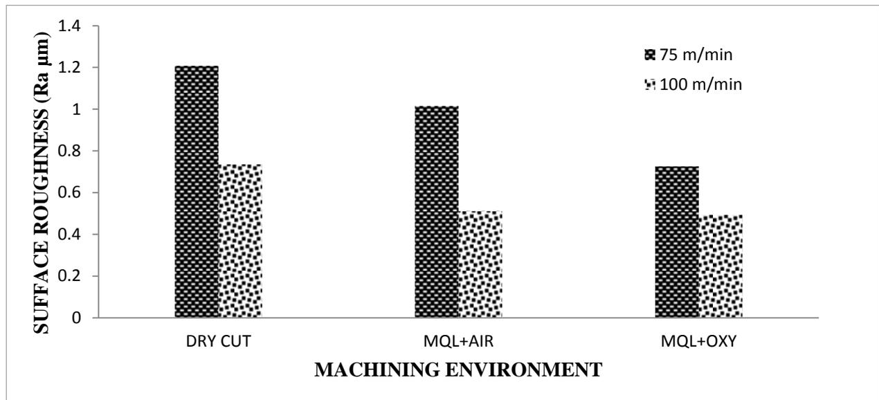
**Figure 4:** Surface roughness Ra ( $\mu\text{m}$ ) vs. machining environment
