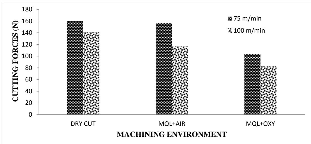
**Figure 5:** cutting forces (N) vs. machining environment
