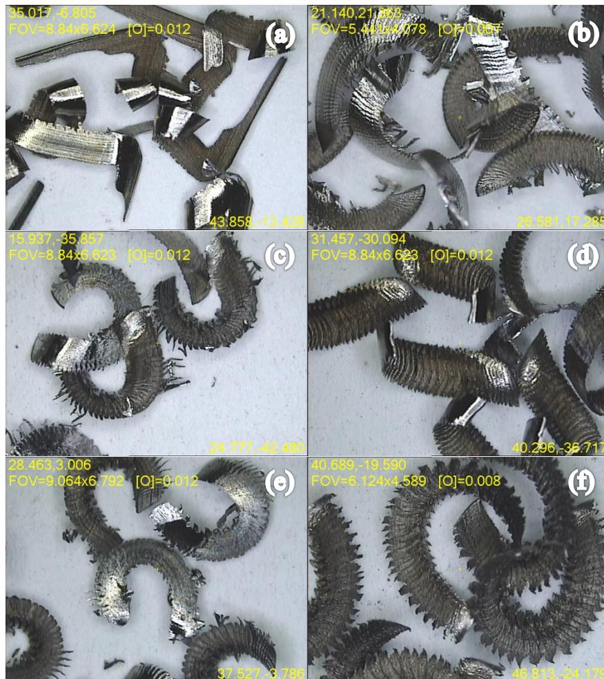
**Figure 7.** Chip morphology under various conditions (a) Dry cut 75m/min (b) Dry cut 100m/min (c) MQL with air 75 m/min (d) MQL with air 100 m/min (e) MQL with oxygen 75 m/min (f) MQL with oxygen 100 m/min.
