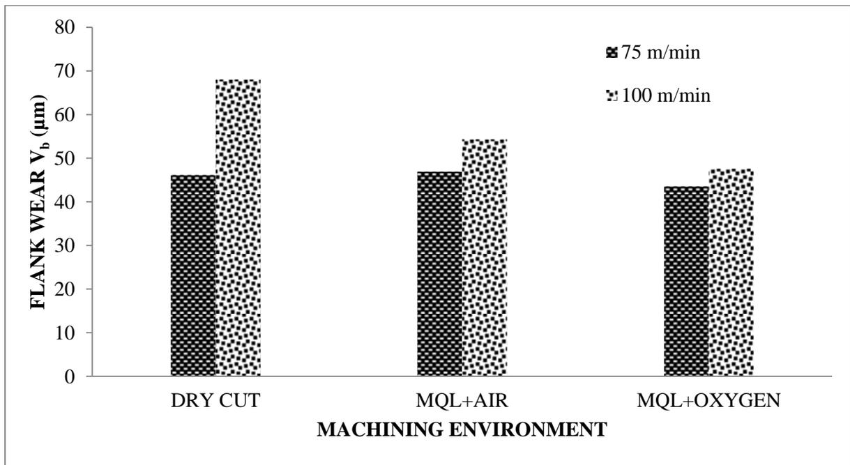
**Figure 2.** Flank wear  $V_b$  ( $\mu\text{m}$ ) with machining environment
