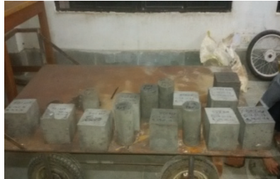
FIGURE 2(a): Hardened concrete
