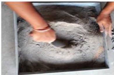
(a) Dry mix of cement with red mud
